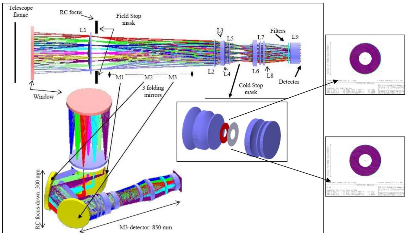
**Figure 4: PANIC optical layout, original (top) and folded (bottom)**
