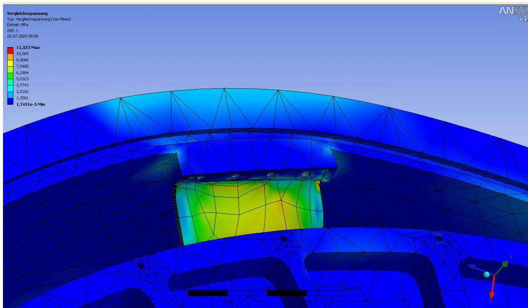
**Figure 56: Finite element simulation of the spacers**
