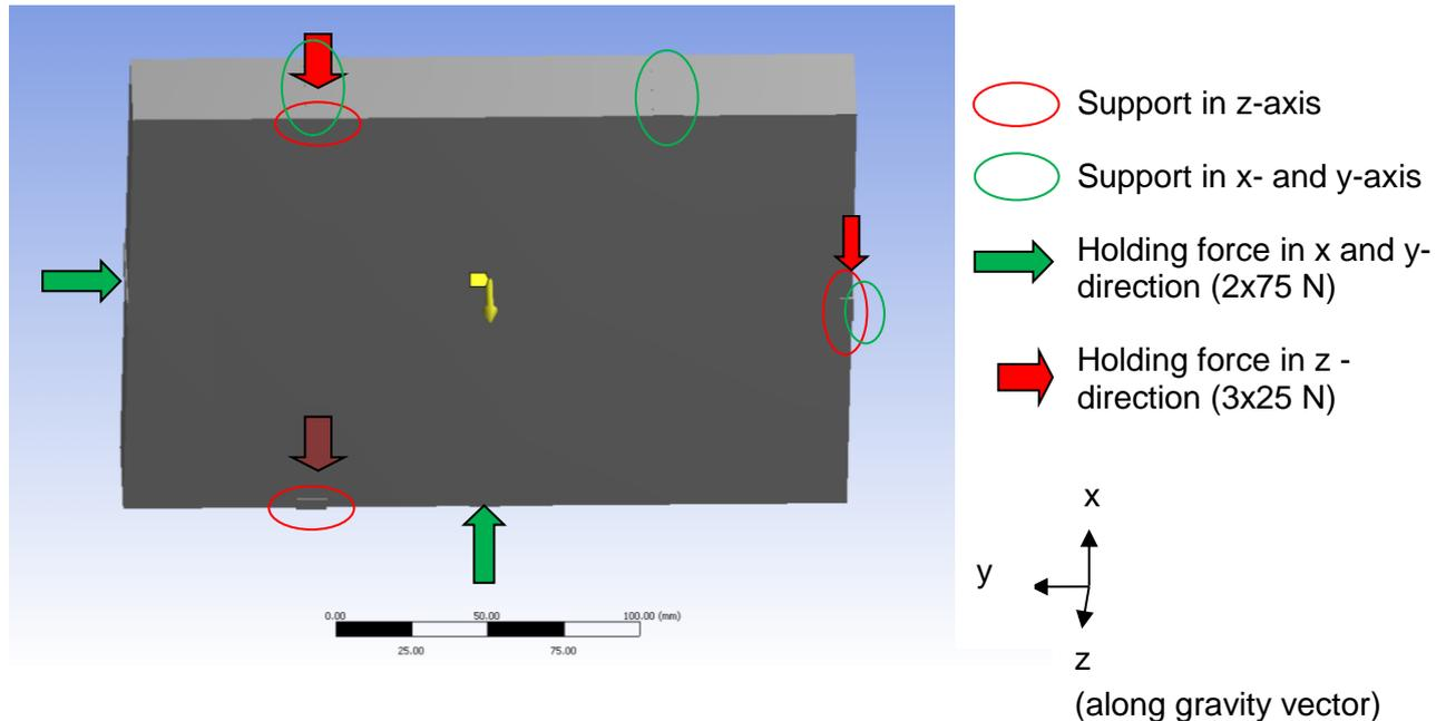
**Figure 23: Boundary conditions to model the mirror support**
