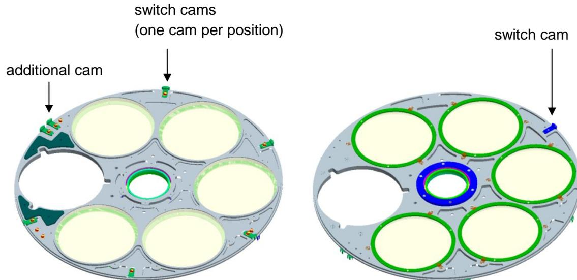
**Figure 46: The filter wheel disc front side (left) has one cam per position, the rear side (right) has only one cam.**
