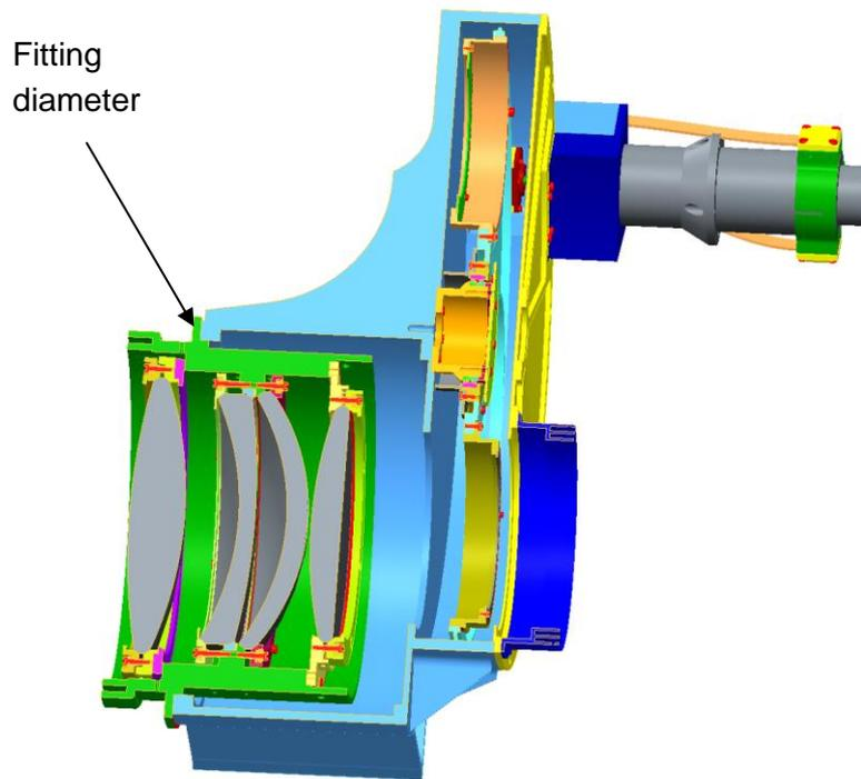
**Figure 26: Positioning of lens mount 2**
