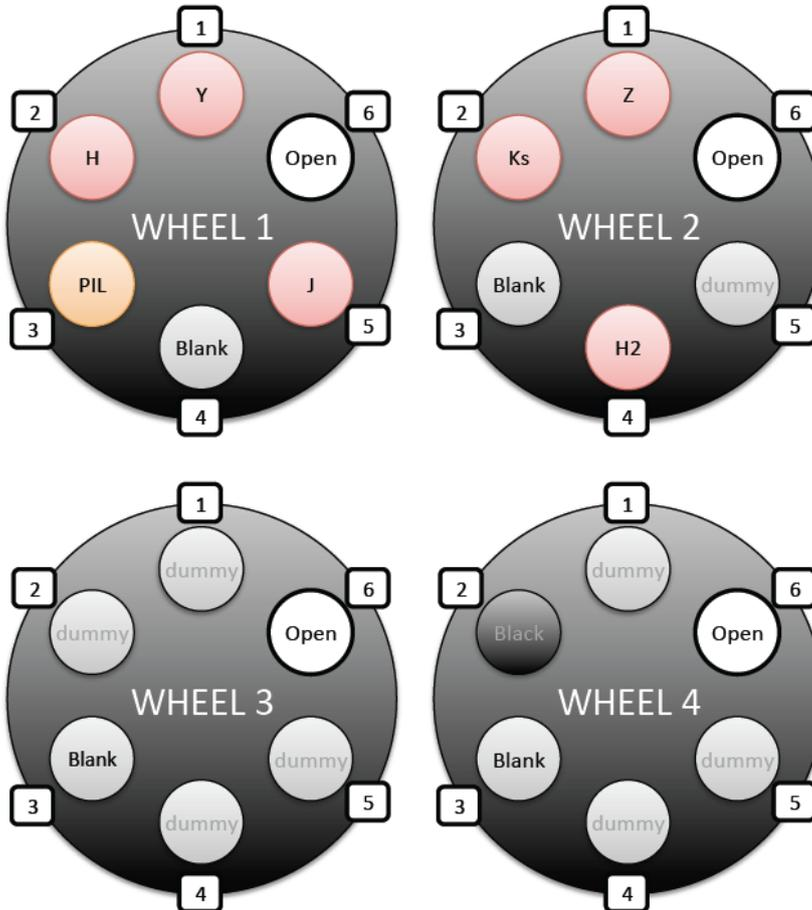
As-built images of the filter wheels. Position 1 is always on top.
