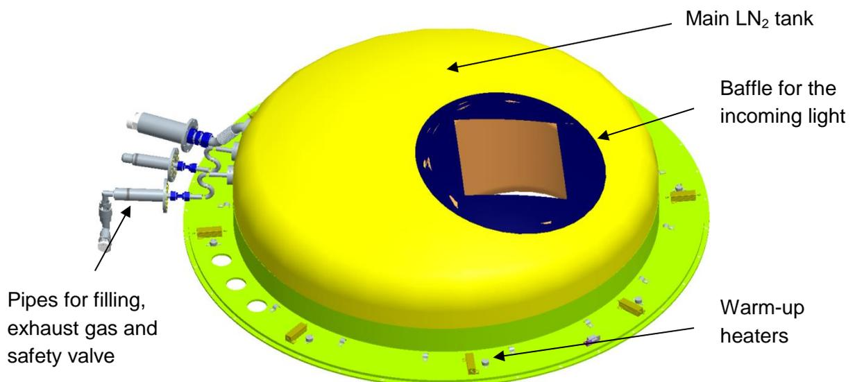
**Figure 50: The main tank subassembly**
