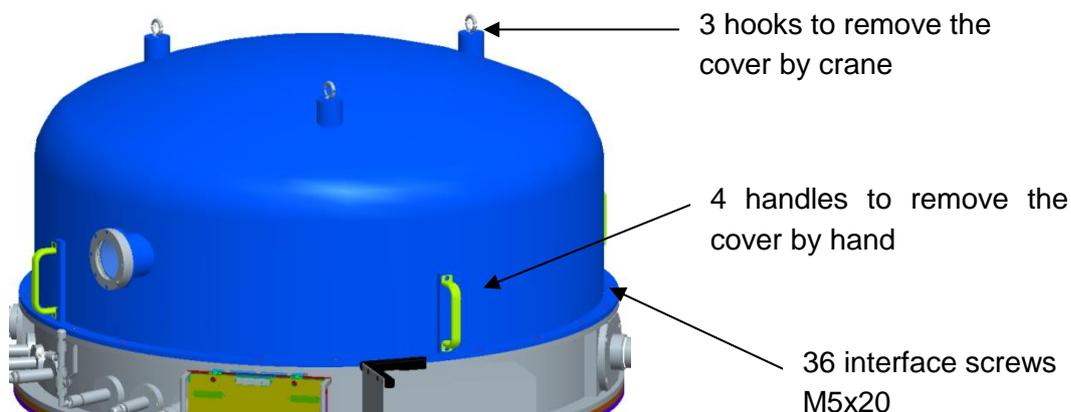
**Figure 62: removing the vacuum cover**
