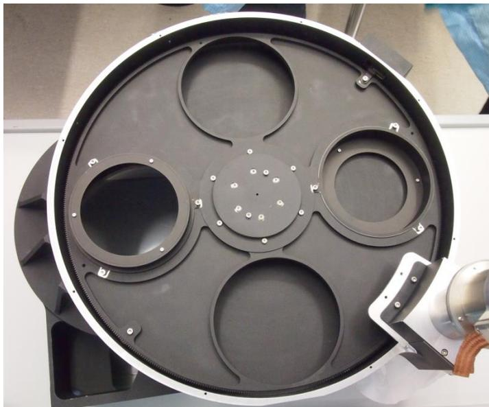
**Figure 31: The cold stop wheel; with cover removed**
