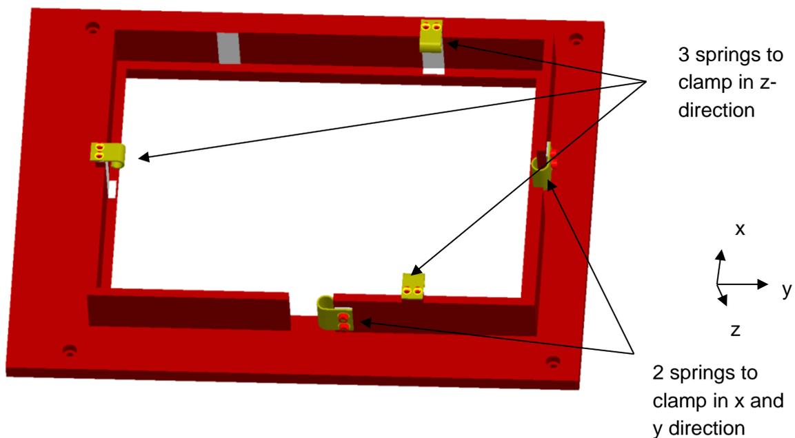
**Figure 22: Mirror holder design for supporting the three mirrors. Three springs clamp the mirror in x direction, one in y and one in z direction.**
