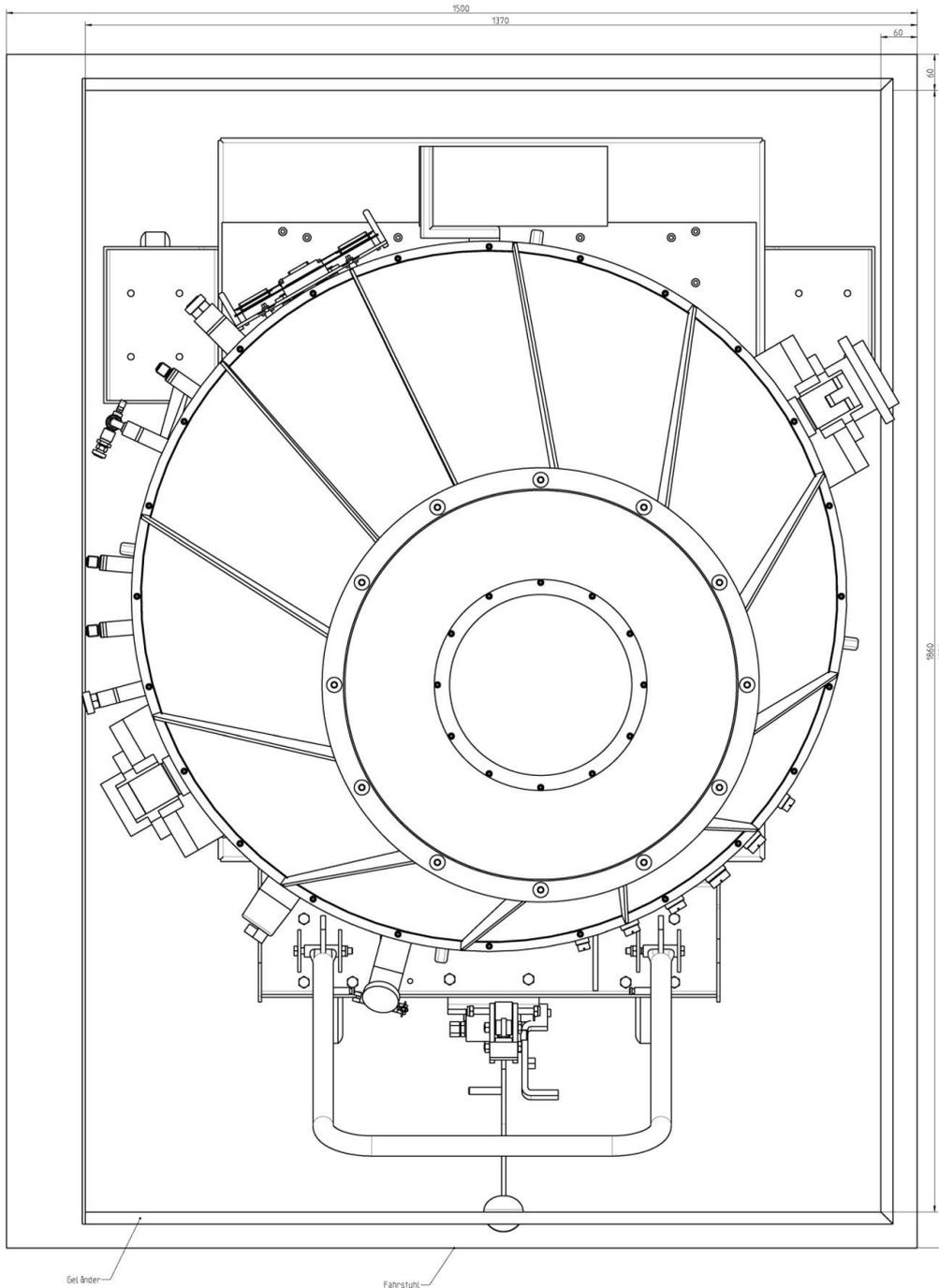
**Figure 81: Cryostat lifting trolley B in 2.2m telescope elevator**
