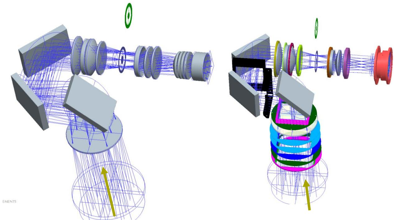
**Figure 7: The optical layout with lenses and mirrors(left) and with baffles (right)**
