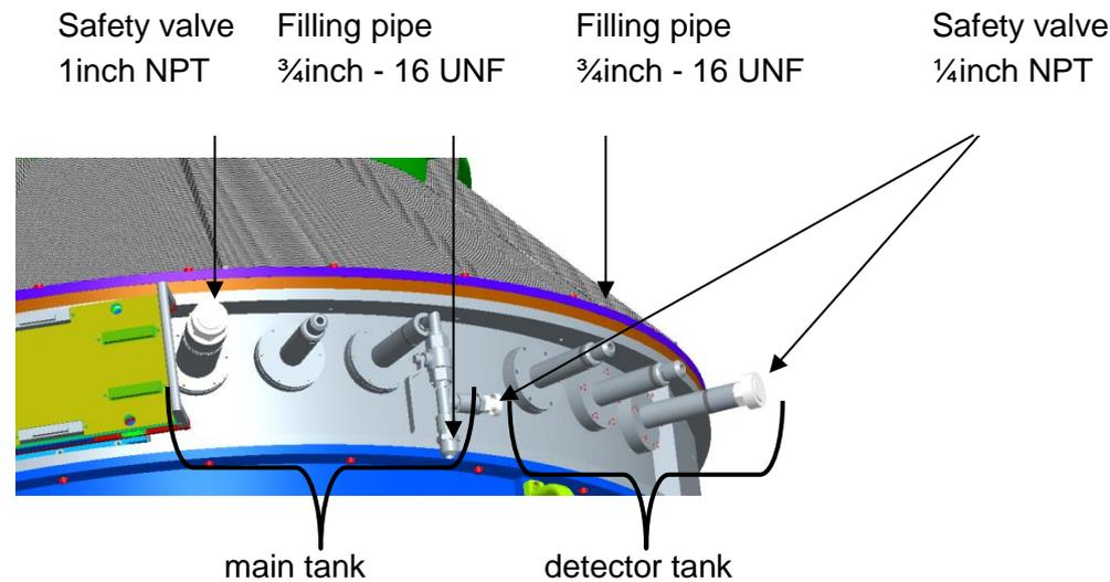
**Figure 65: Connections to the tanks for the cryogenic liquids**
