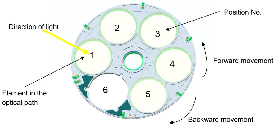
**Figure 43: Definition of wheel positions and directions**
