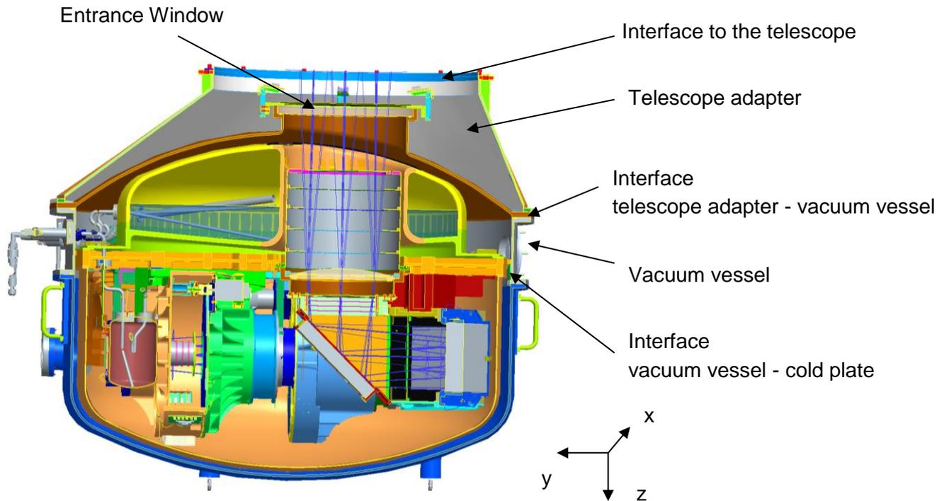
**Figure 11: Interfaces and components included in "complete optics"**
