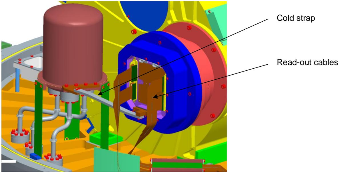
**Figure 73: Detector assembly**
