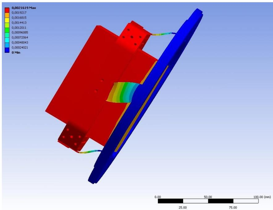
**Figure 72: FE-Simulation due to self weight deflection of the detector mount**
