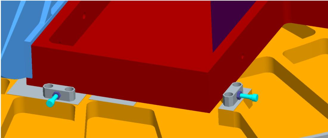
**Figure 16: Adjustment screws allow optics mount 1 to be shifted in x and y direction.**
