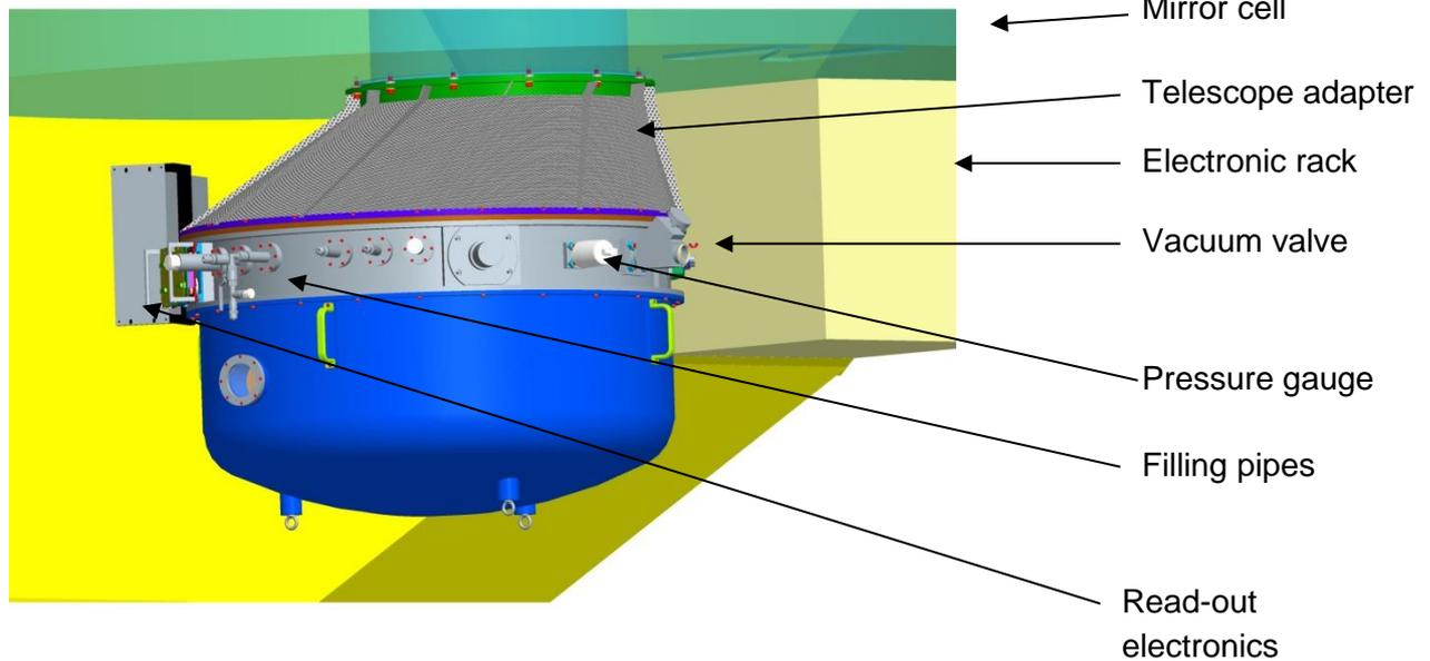
**Figure 3: PANIC at the 2.2m telescope**
