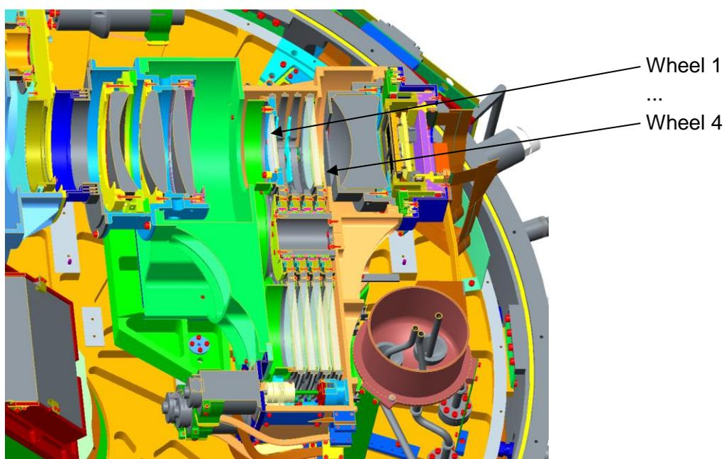
**Figure 37: The wheels are numbered according to their order in the light-path**
