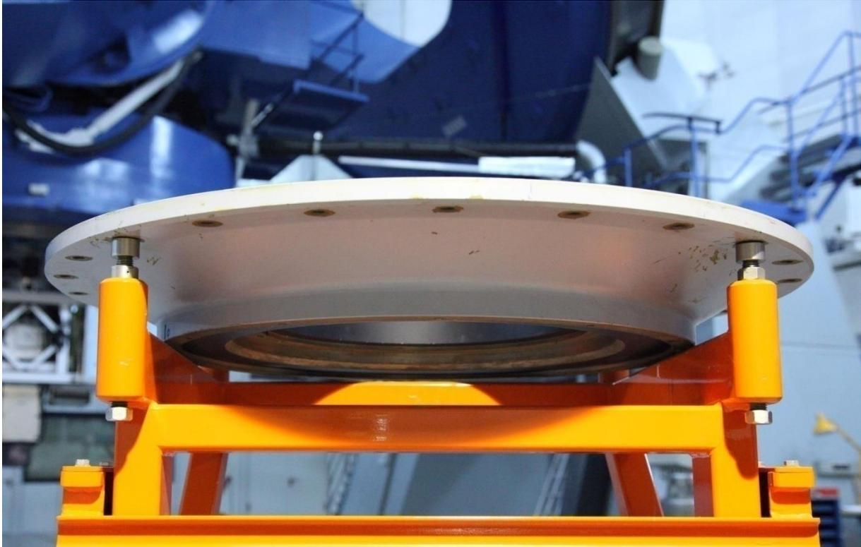
**Figure 69: An adapter flange allows instruments designed for the 2.2 m telescope to be used at the 3.5 m telescope**
