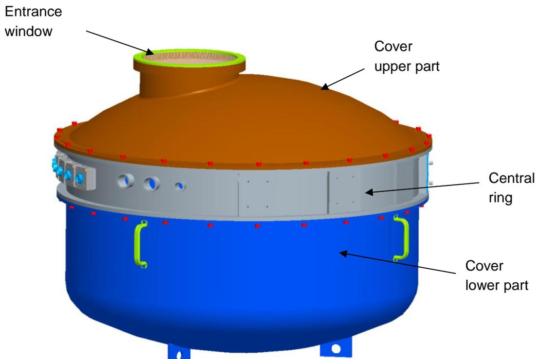
Figure 48: The vacuum vessel.
