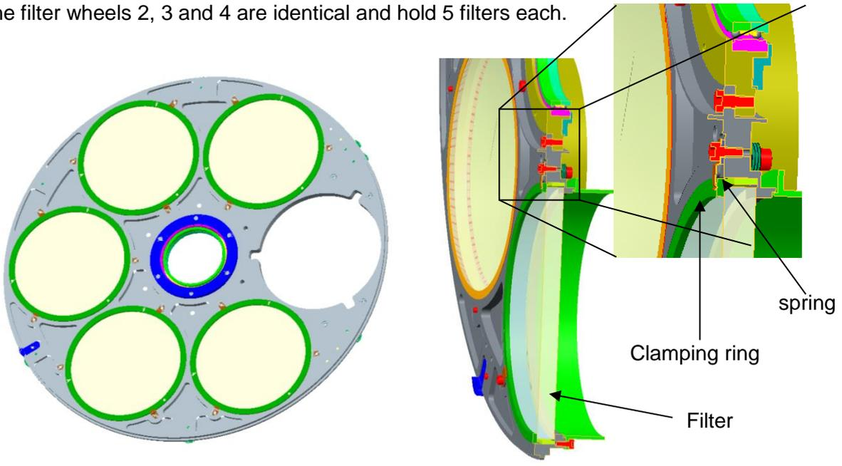
**Figure 39: Left: Design of the filter wheels 2 - 4. Right: Cross section showing mounting concept.**
