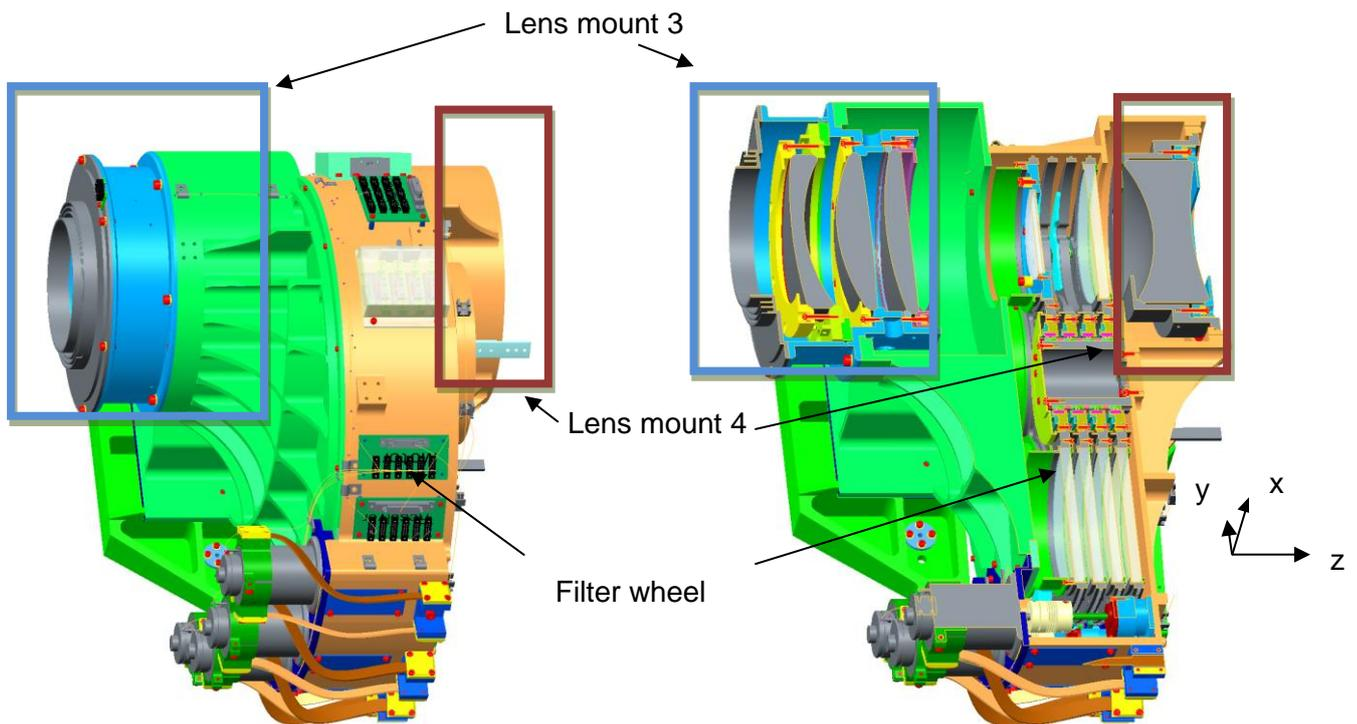
**Figure 33: Optics mount 2 and its components**
