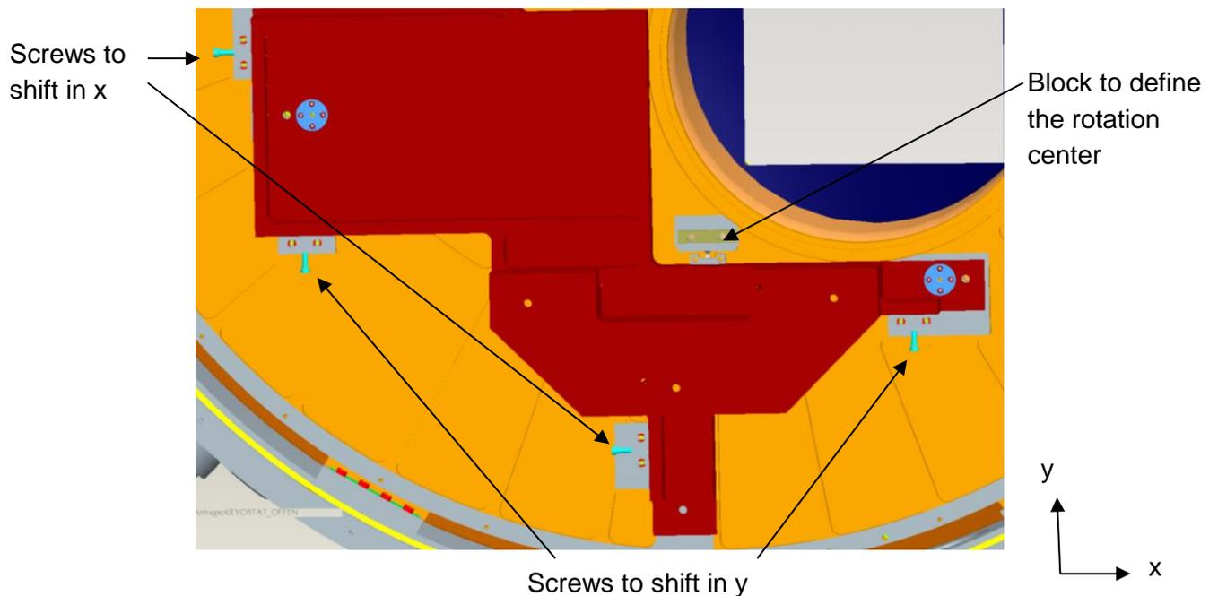
**Figure 17: Optics mount 1 adjustment principle**
