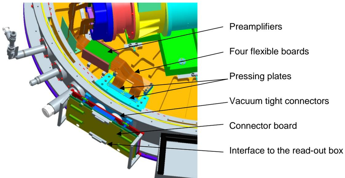
**Figure 58: Feedthroughs for the detector read-out.**
