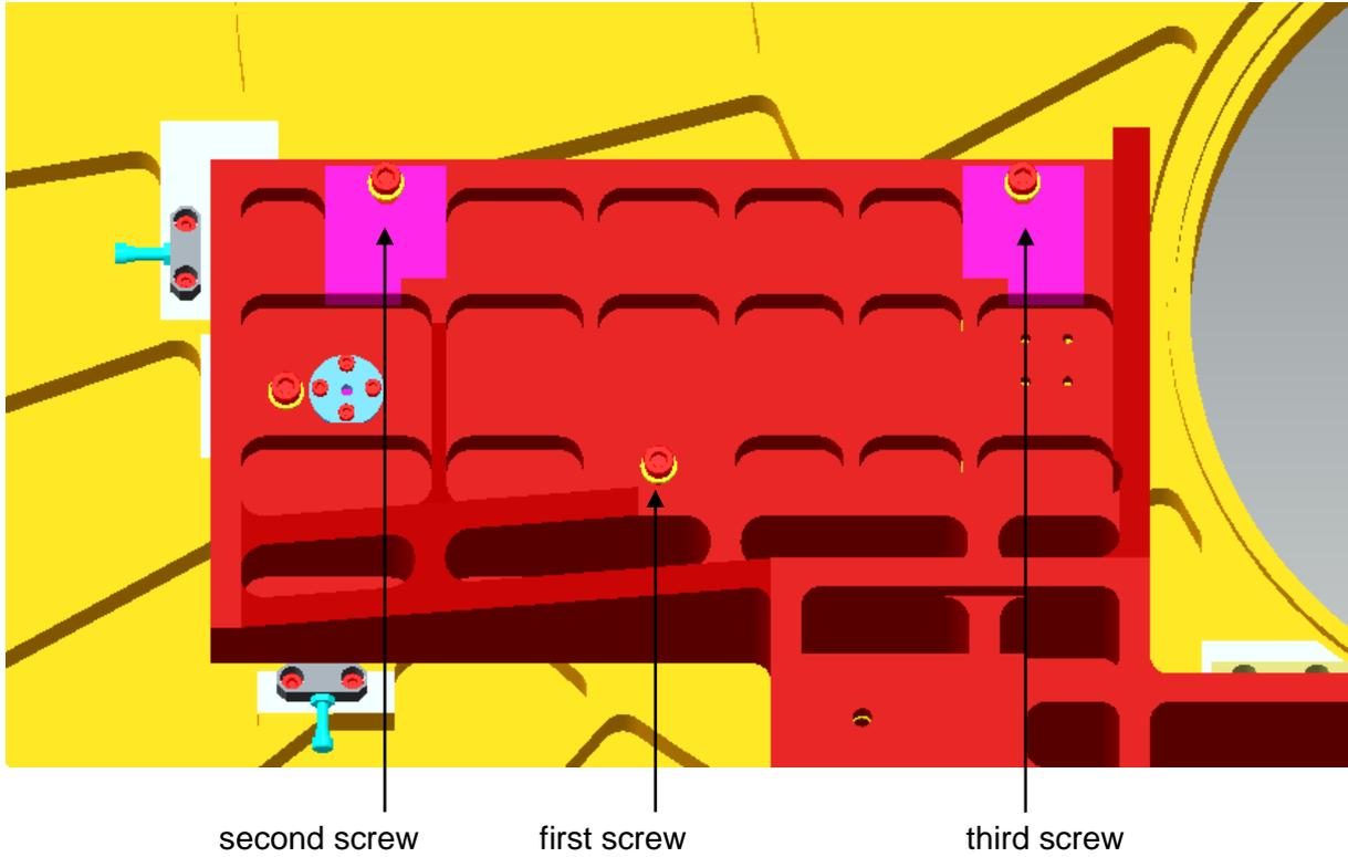
**Figure 32: Sequence to tighten the screws of Cold Stop Wheel**
