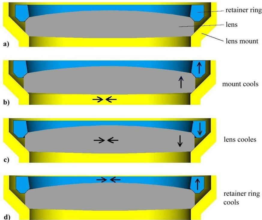
**Figure 10: Displacements of lens and retainer ring due to thermal shrinkage while cooling down (explanation in the text)**
