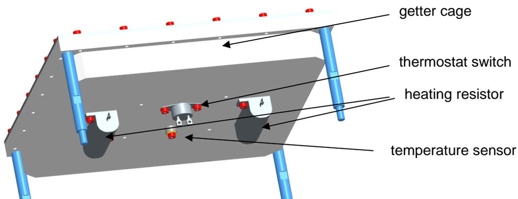
**Figure 61: Two heaters, a thermostat switch and a temperature sensor are used to control the temperature of the getter cage**
