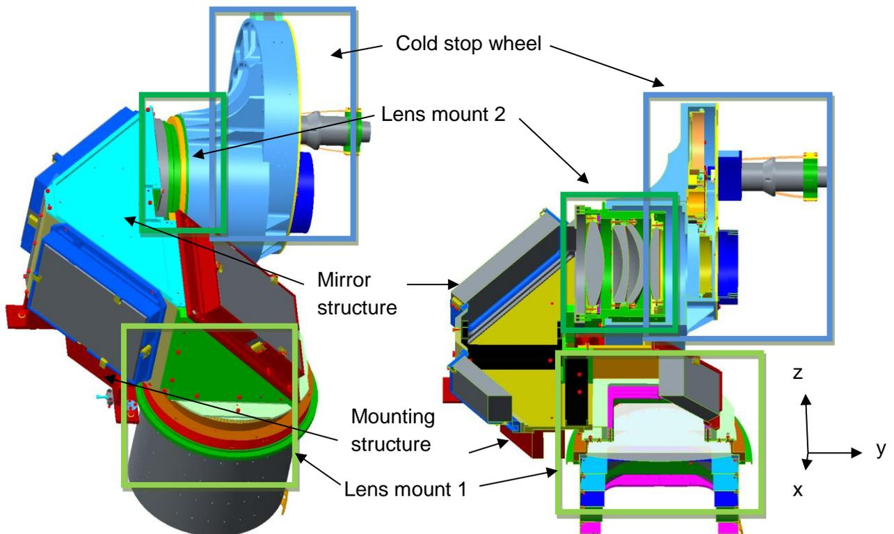
**Figure 14: Optics mount 1 and its sub-components**
