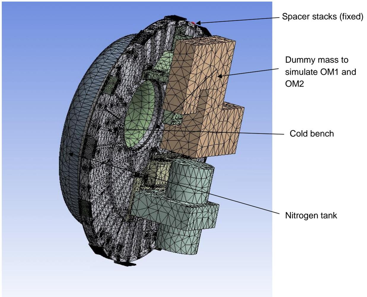
**Figure 12: Simulation of the cold bench including the dummy masses.**
