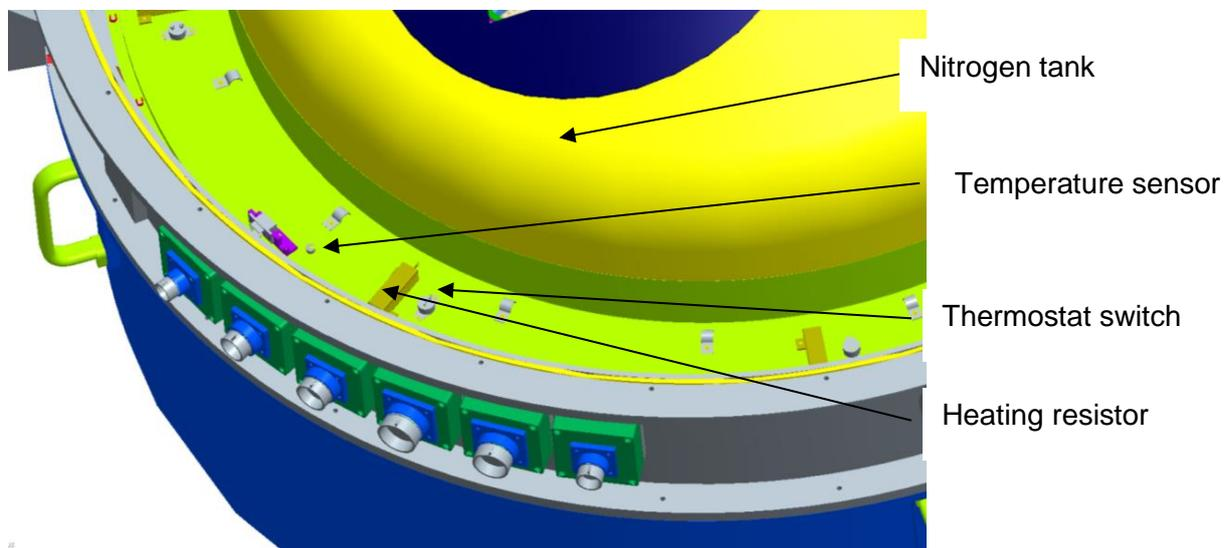
**Figure 60: Eight heaters in two circuits attached to the nitrogen tank are used to warm-up PANIC**
