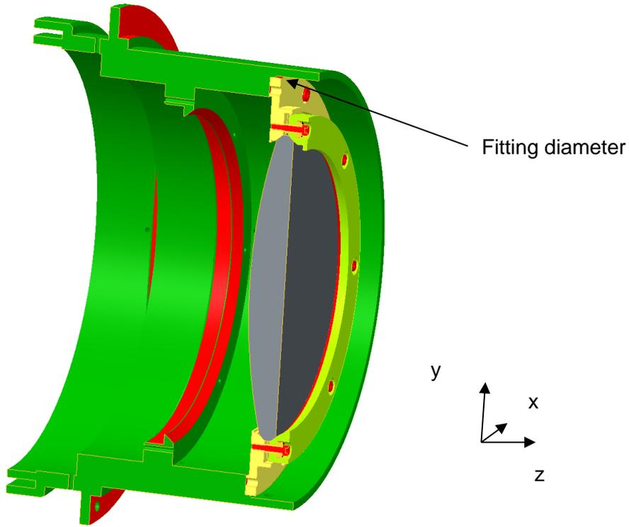
**Figure 29: Lens 5 with its support in Lens Mount 2**
