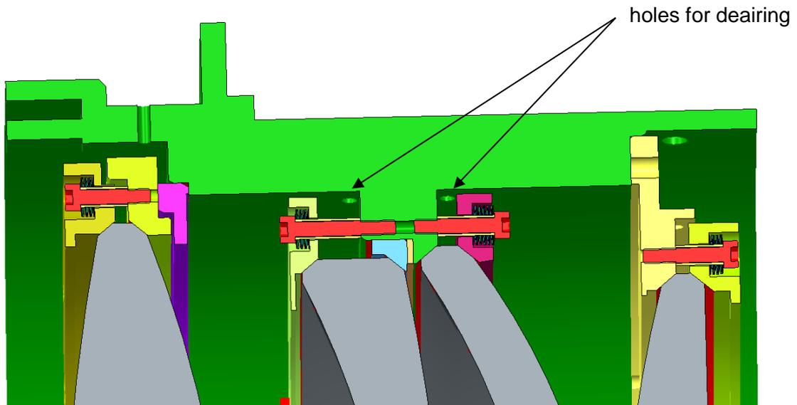
**Figure 25: De-airing is done by radial holes**
