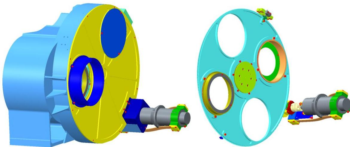
**Figure 30: The cold stop wheel; left the complete view right without cover**
