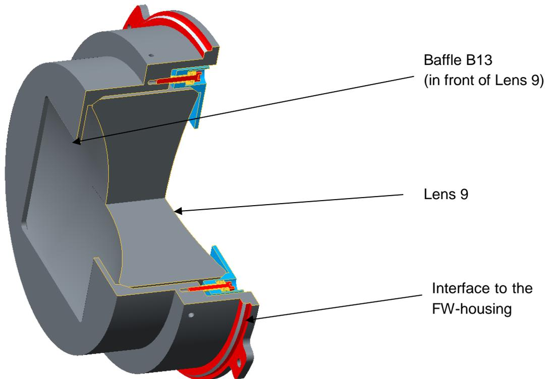
**Figure 41: Lens mount 4 with lens 9 attached.**
