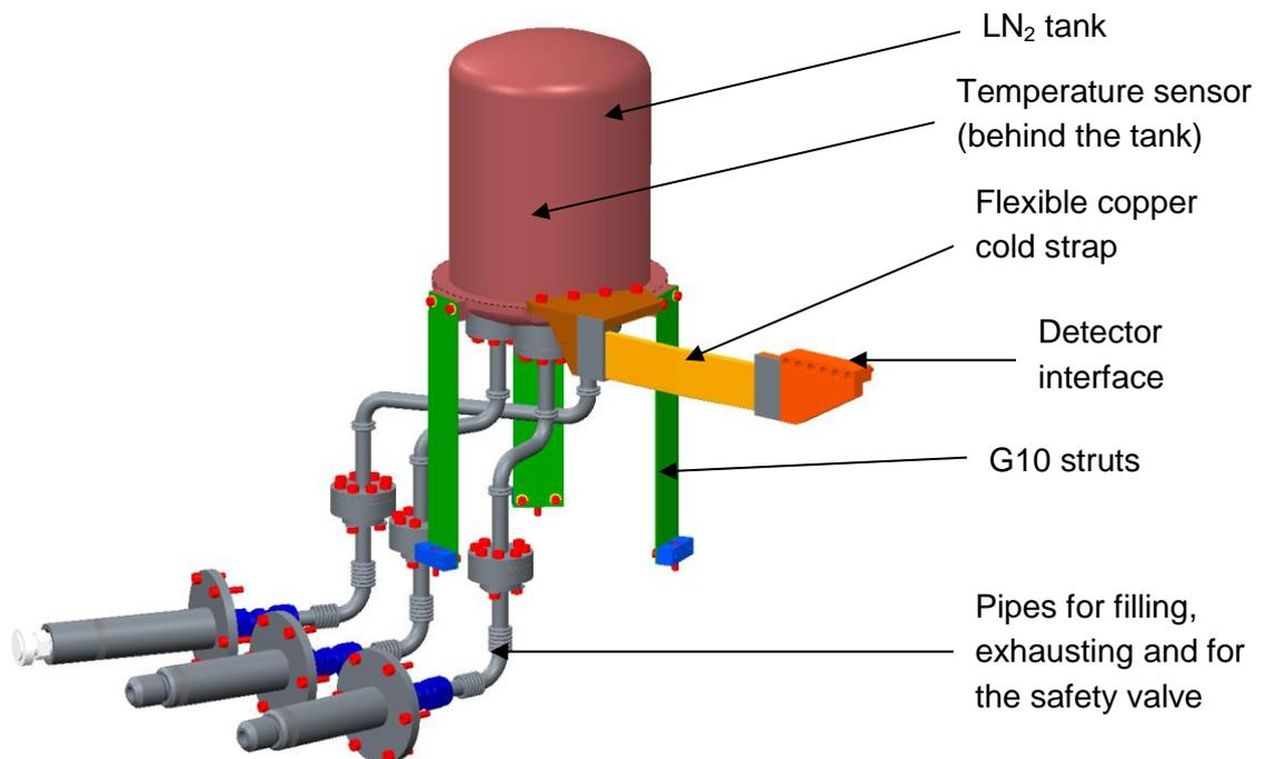
**Figure 53: The detector tank subassembly**
