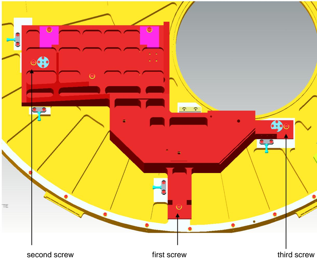
**Figure 18: Sequence to tighten the screws of OM1**
