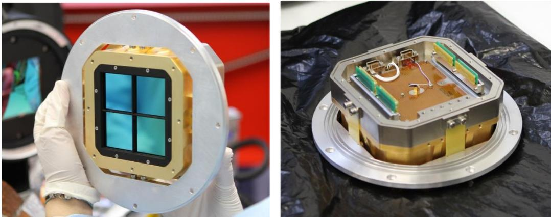
**Figure 5: The focal plane array. The greenish areas are the 4 light sensitive areas (left). The back of the module with connectors and heaters (right)**
