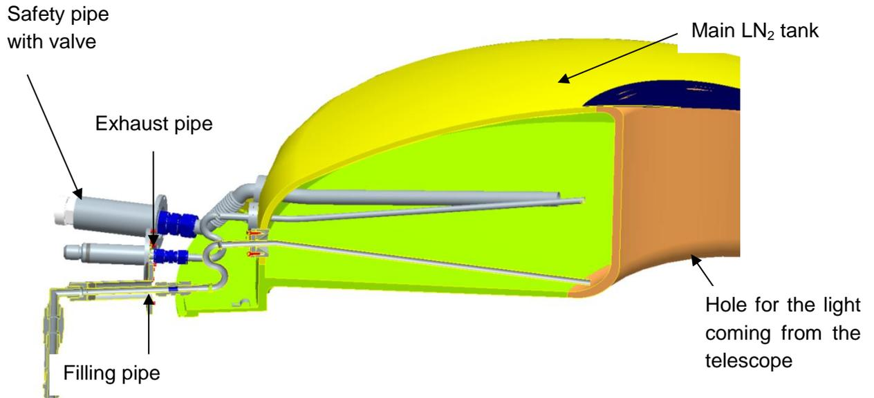
**Figure 51: Cross section through the main tank showing the connecting pipes**
