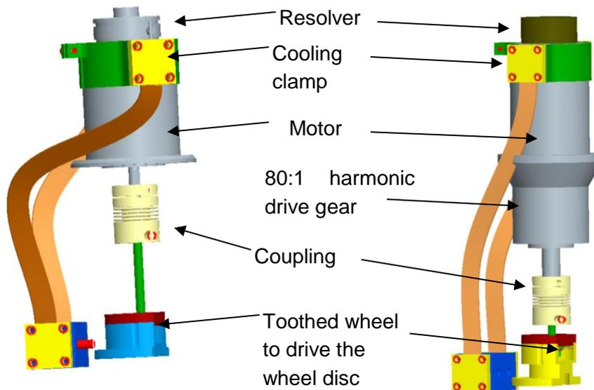
**Figure 44: The main parts of the wheel drives. Left: one of four identical filter wheel power trains, right: the power train for the cold stop wheel**
