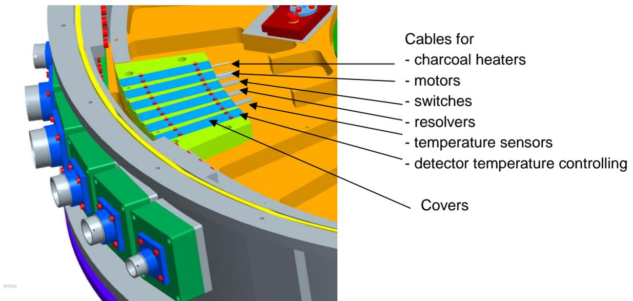
**Figure 57: Feedthroughs for the cryostat cabling**
