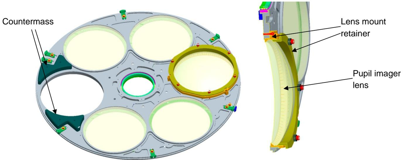
**Figure 38: Filter wheel 1 with the pupil imager lens and counterweights**
