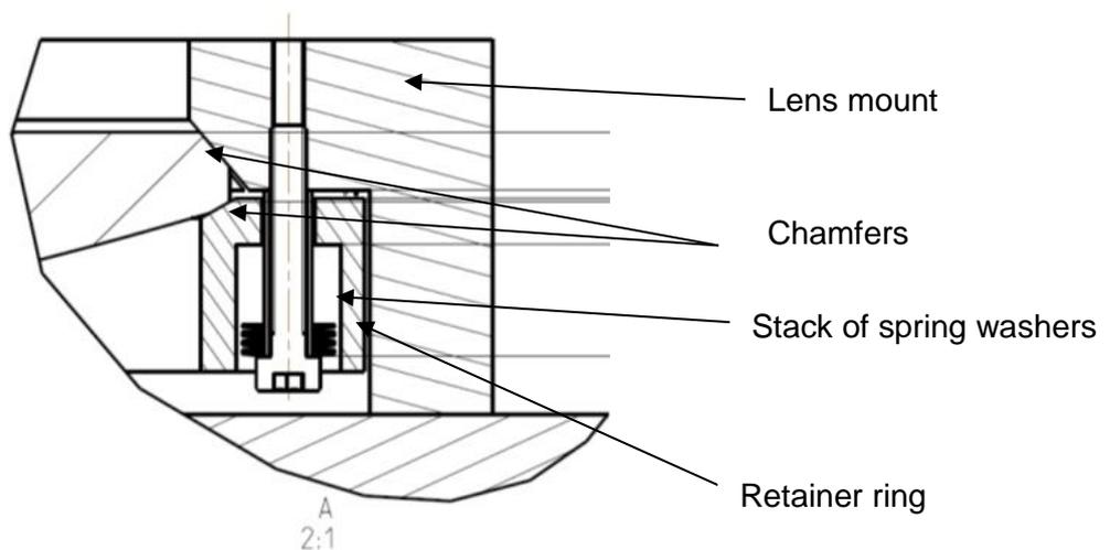
Figure 9: Cross-sectional view through the lens alignment design (explanation in the text)
