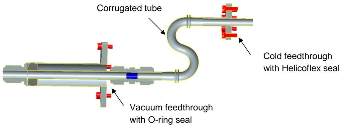
**Figure 52: Cross section through the exhaust pipe**
