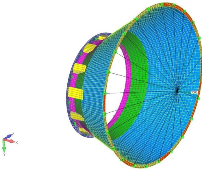
**Figure 68: FE-Model of the telescope adapter**
