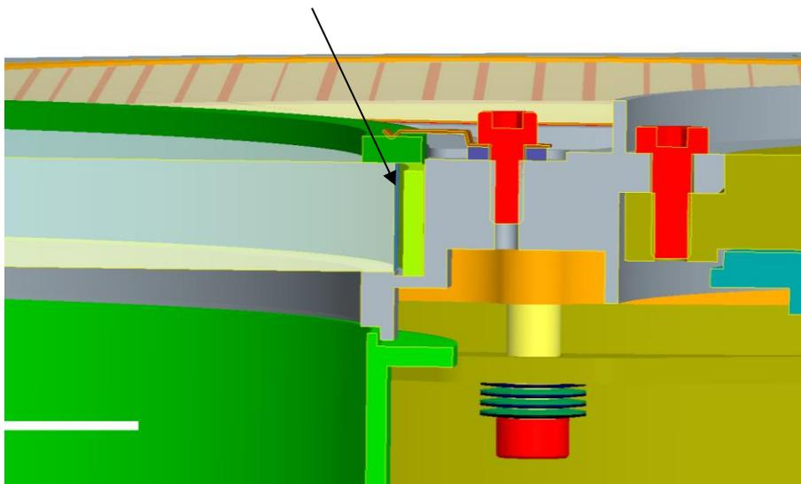
The inner diameter of this ring is large enough to ensure a gap to the filters of 0.5mm at cold. Assuming the FSi substrate does not shrink at all and remains at 117.855 mm in diameter, the inner diameter of the ring has a diameter of 119.4 mm at warm resulting in 118.95 mm at cold. The resulting gap will be 0.55 mm.
