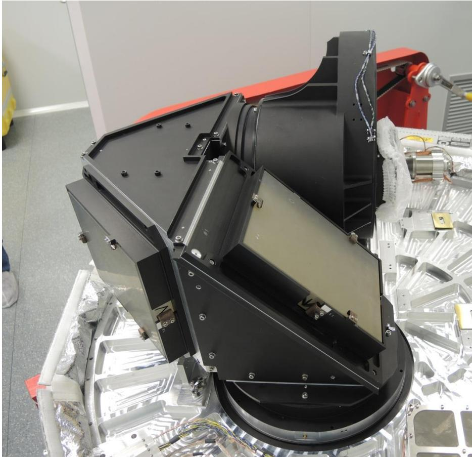
**Figure 15: Optics mount 1 after installation into the cryostat**
