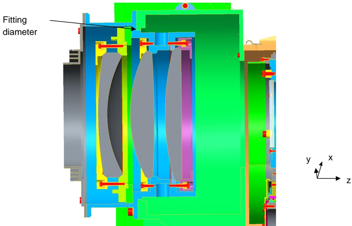
**Figure 36: Positioning of lens mount 3**
