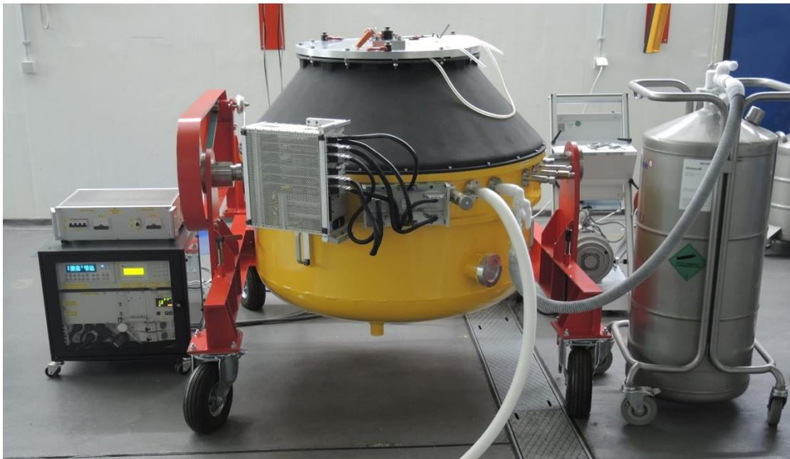
**Figure 1: PANIC cryostat in its caddy with control and read-out electronics, the conical telescope adapter, the crane-flange and a liquid nitrogen vessel for filling.**
