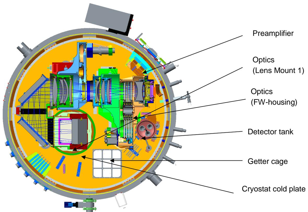
**Figure 59: Distribution of the temperature sensors inside the PANIC cryostat. Not shown are the sensors on the LN<sub>2</sub> main tank, on the shield and inside the detector module.**
