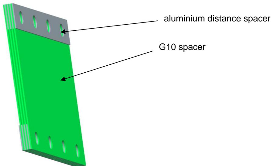
**Figure 55: Stack of G10 spacers. Four spacers form a stack at PANIC**
