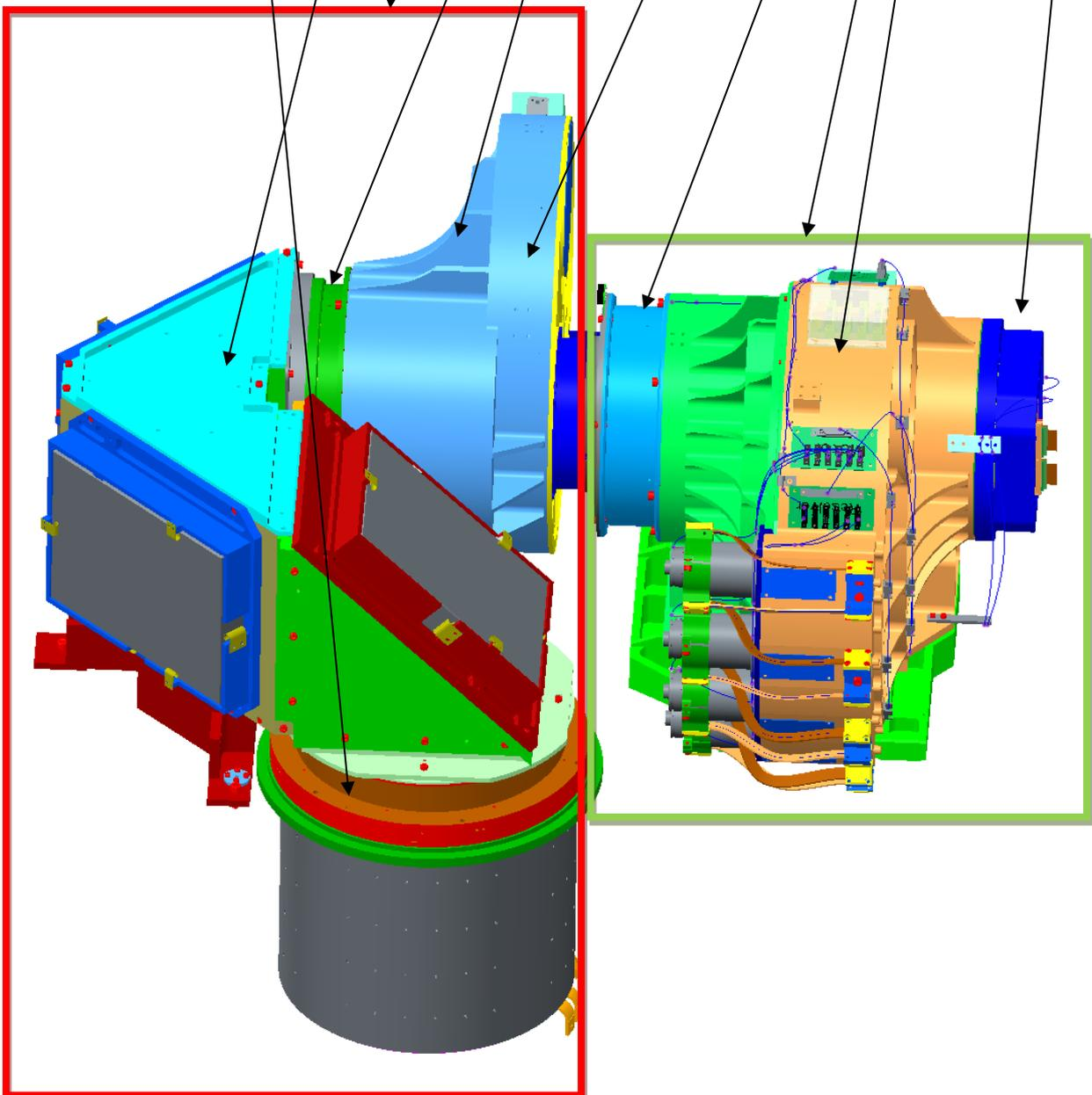
Figure 8: Overview over the optical elements and their mounts
