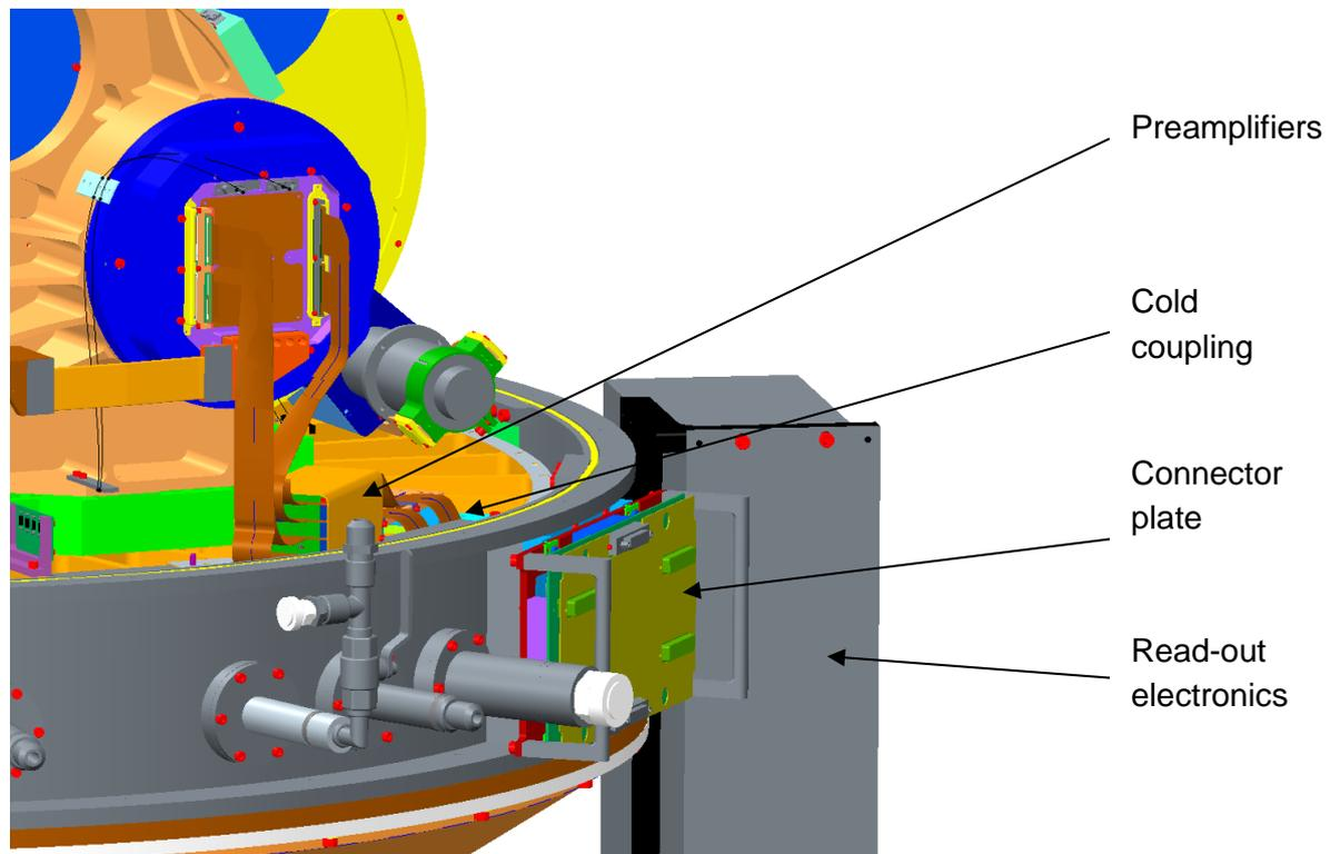
**Figure 74:Read-out cabling**
