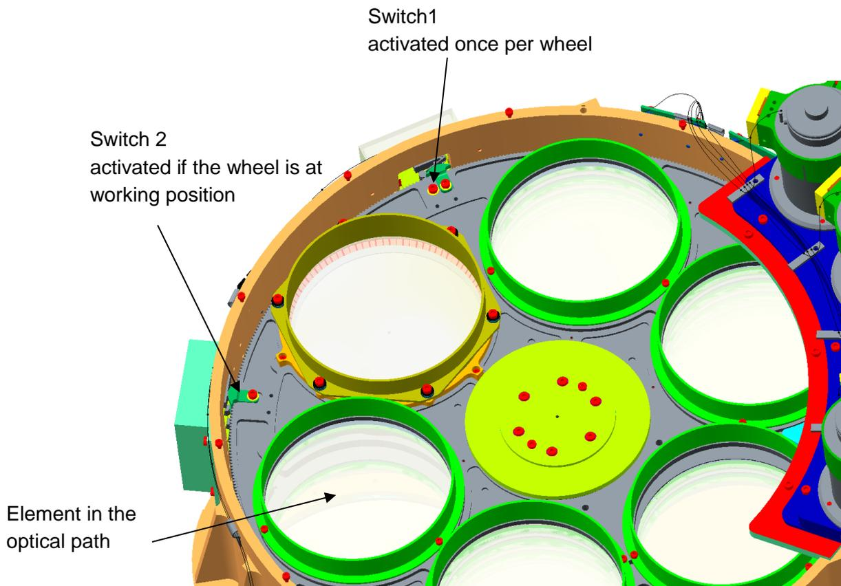
**Figure 45: Two switches per wheel provide information about the actual wheel position**
