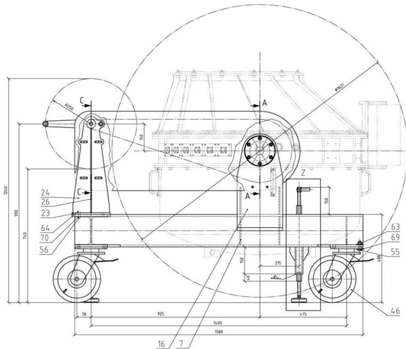
**Figure 76: Dimensions of trolley A**
