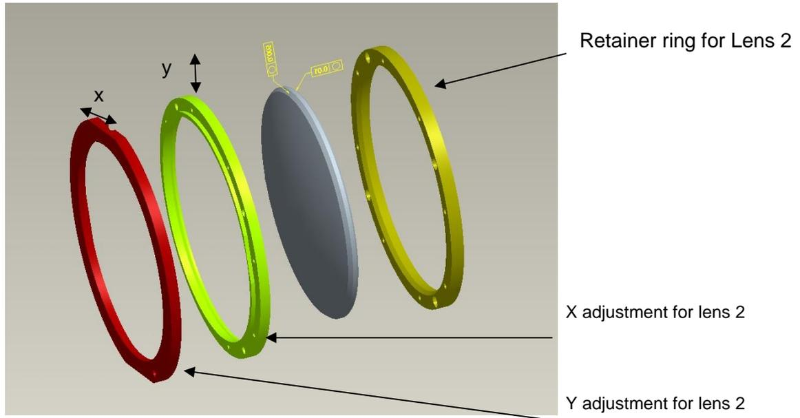
**Figure 27: Adjustment unit for Lens 2**
