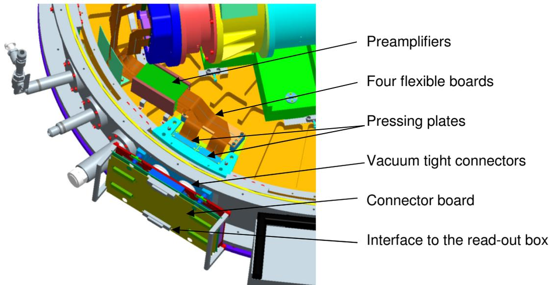
**Figure 56: Feedthroughs for the detector read-out.**
