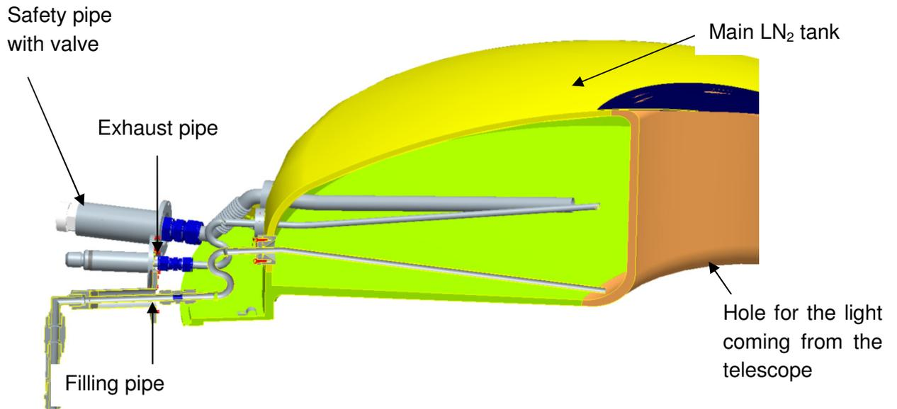
**Figure 49: Cross section through the main tank showing the connecting pipes**
