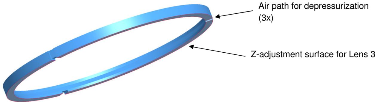
**Figure 28: Adjustment ring for lens 3**
