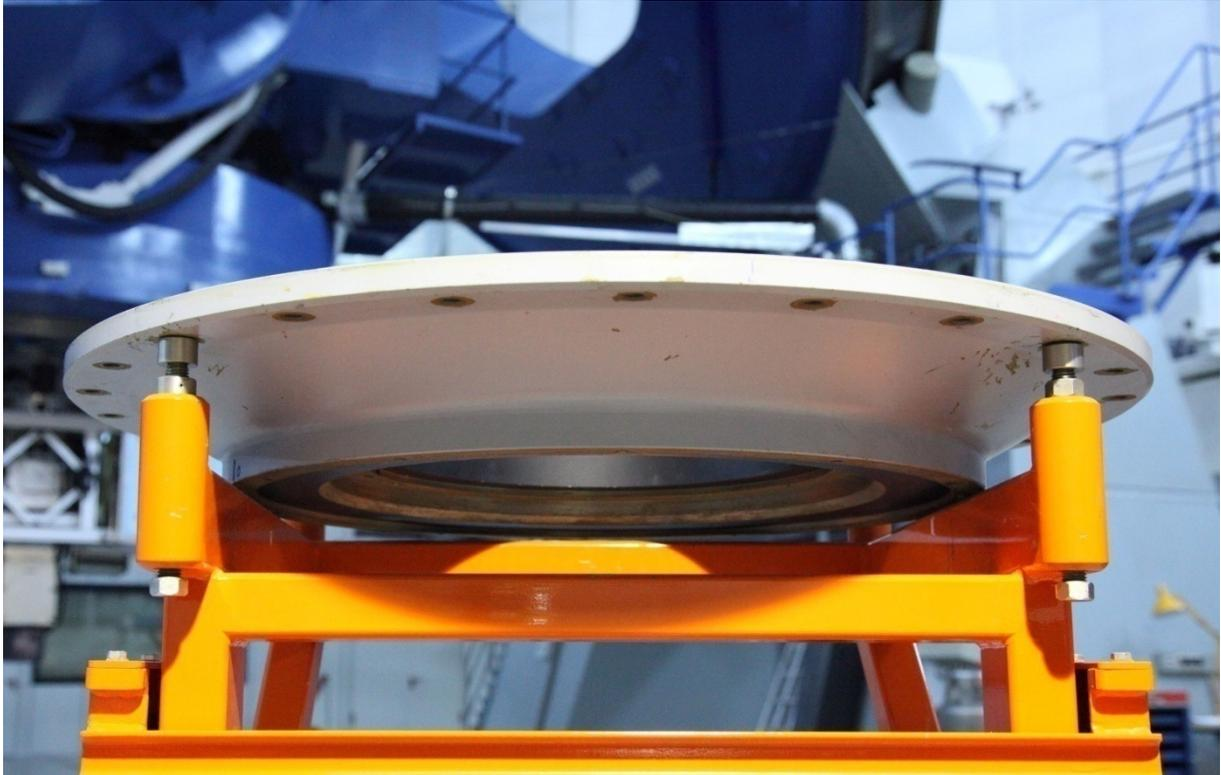
**Figure 67: An adapter flange allows instruments designed for the 2.2 m telescope to be used at the 3.5 m telescope**
