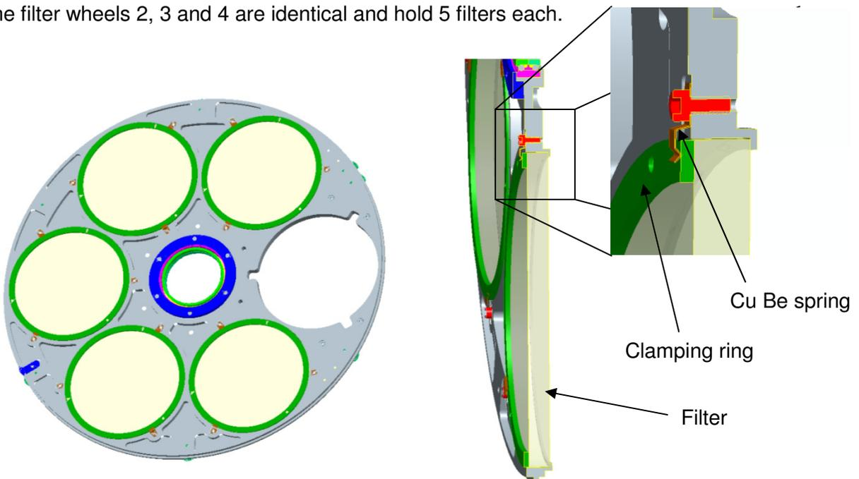
**Figure 36: Left: Design of the filter wheels 2 - 4. Right: Cross section showing mounting concept.**
