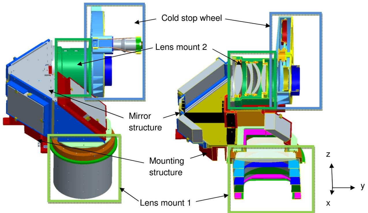
**Figure 16: Optics mount 1 and its sub-components**
