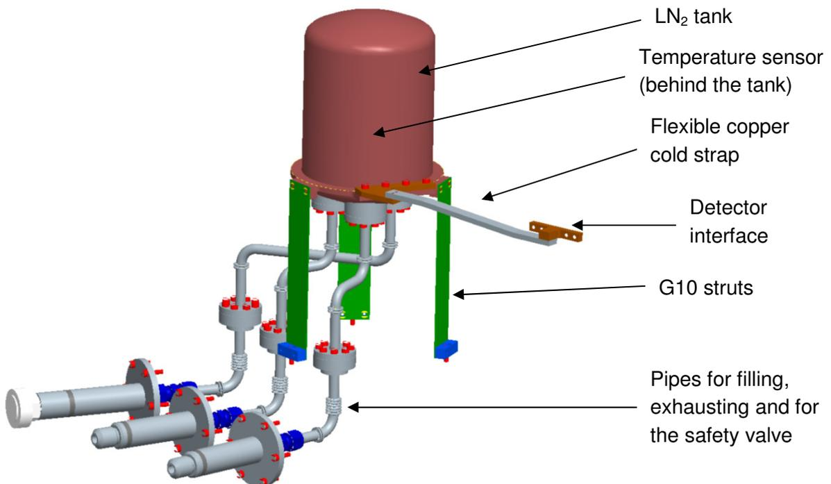
**Figure 51: The detector tank subassembly**
