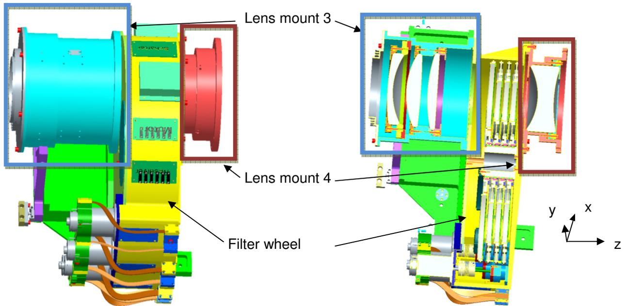
**Figure 31: Optics mount 2 and its components**
