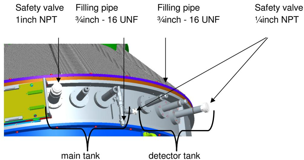
**Figure 63: Connections to the tanks for the cryogenic liquids**
