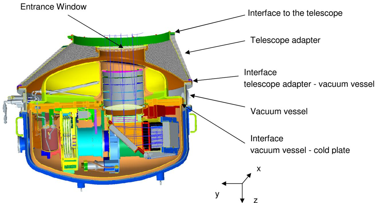
**Figure 13: Interfaces and components included in "complete optics"**
