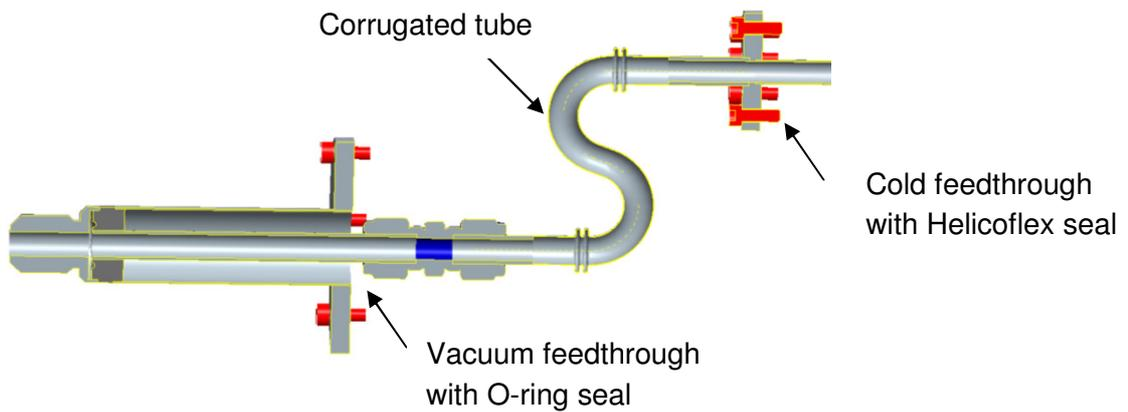
**Figure 50: Cross section through the exhaust pipe**
