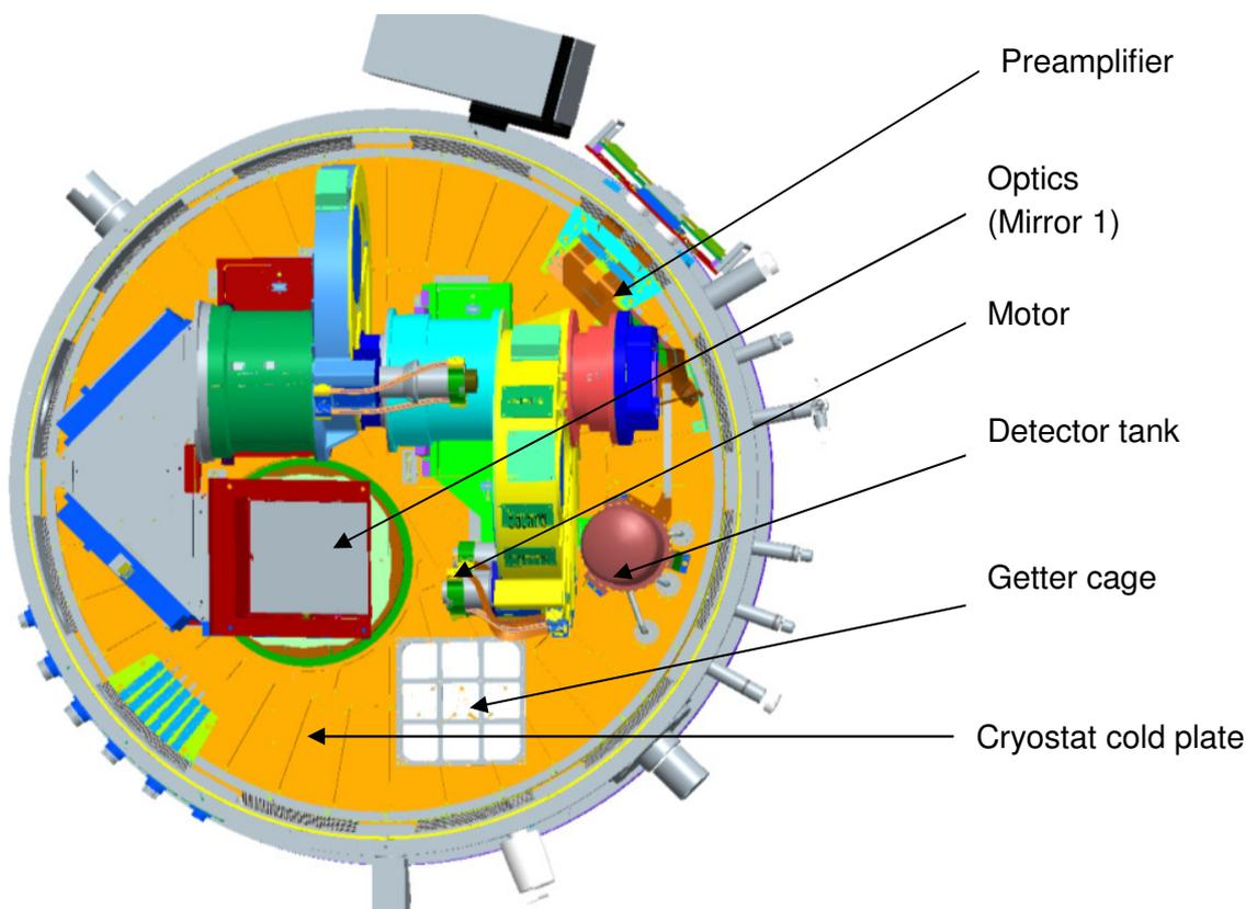
**Figure 57: Distribution of the temperature sensors inside the PANIC cryostat. Not shown are the sensors on the LN<sub>2</sub> main tank, on the shield and inside the detector module.**
