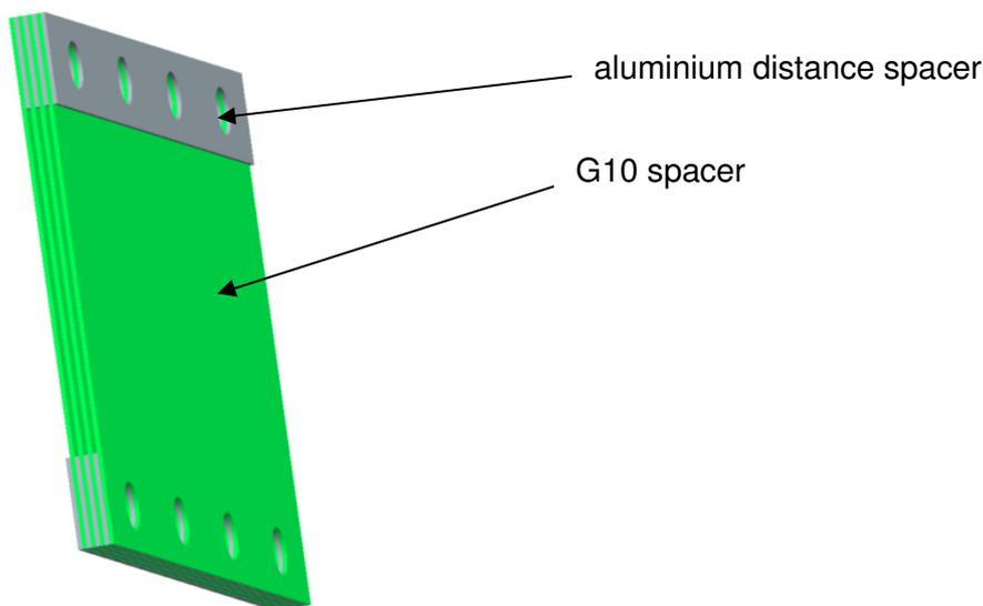
**Figure 53: Stack of G10 spacers. Four spacers form a stack at PANIC**
