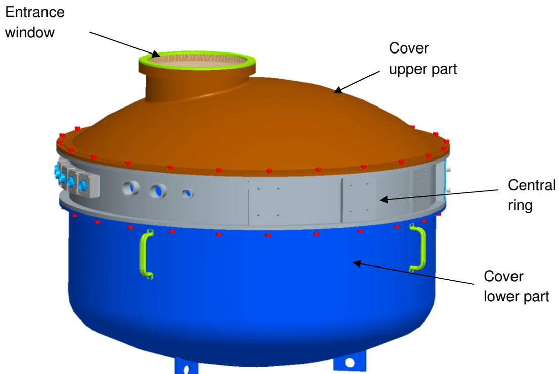
Figure 46: The vacuum vessel.
