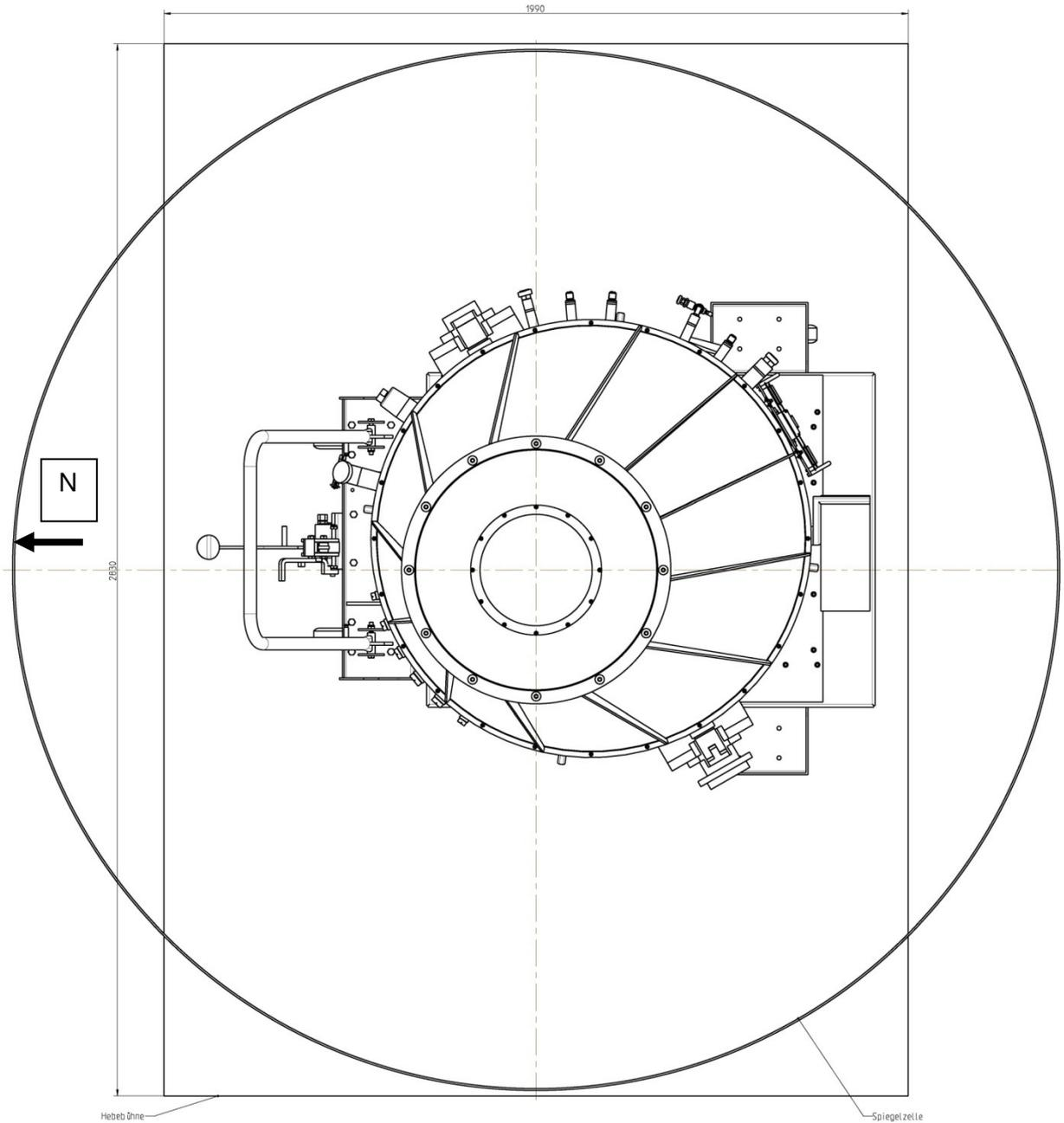
**Figure 78: PANIC with reference to the 2.2m-telescope mirror and the instrument lifting platform**
