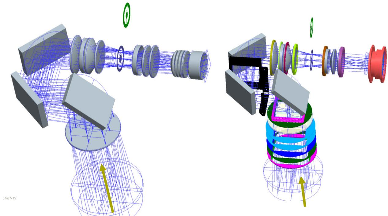
**Figure 8: The optical layout with lenses and mirrors(left) and with baffles (right)**
