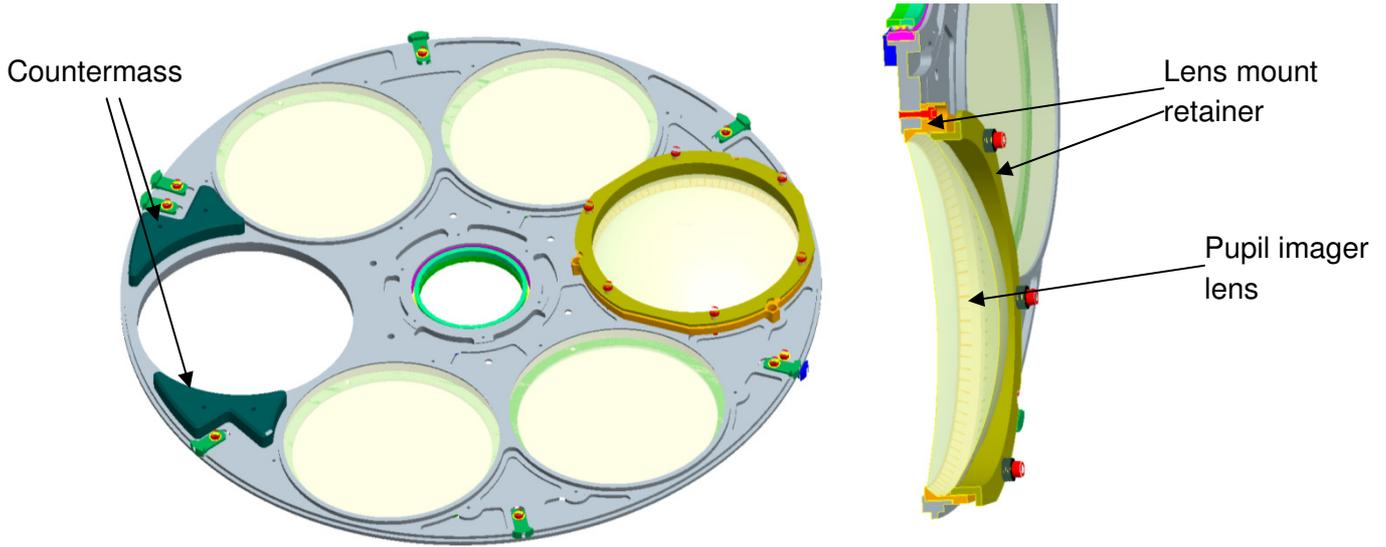
**Figure 35: Filter wheel 1 with the pupil imager lens and counterweights**
