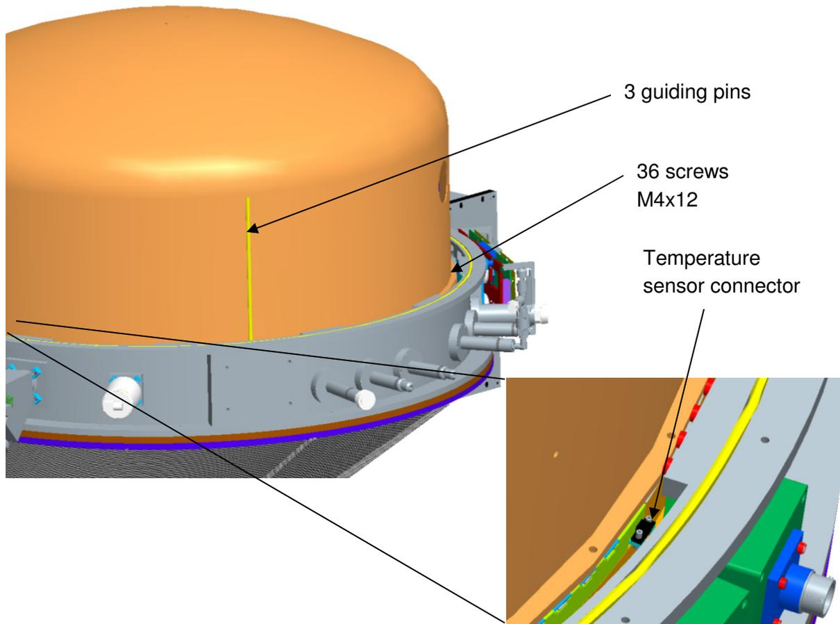
**Figure 61: removing the nitrogen shield**
