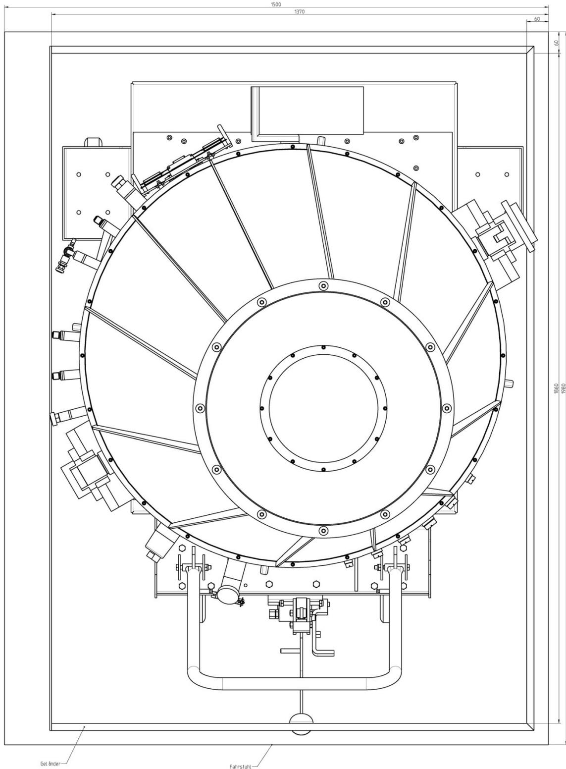
**Figure 77: Cryostat lifting trolley B in 2.2m telescope elevator**
