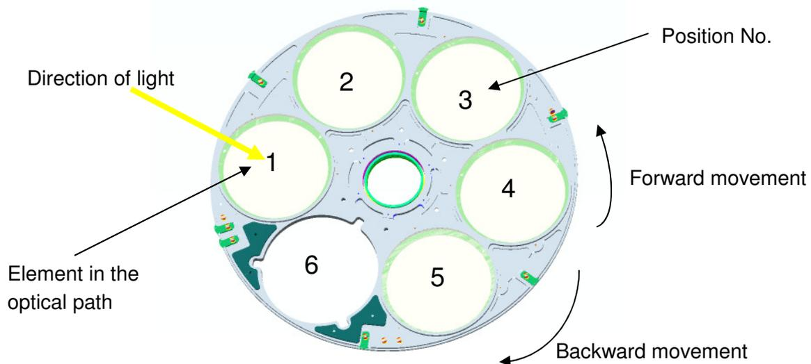
**Figure 41: Definition of wheel positions and directions**
