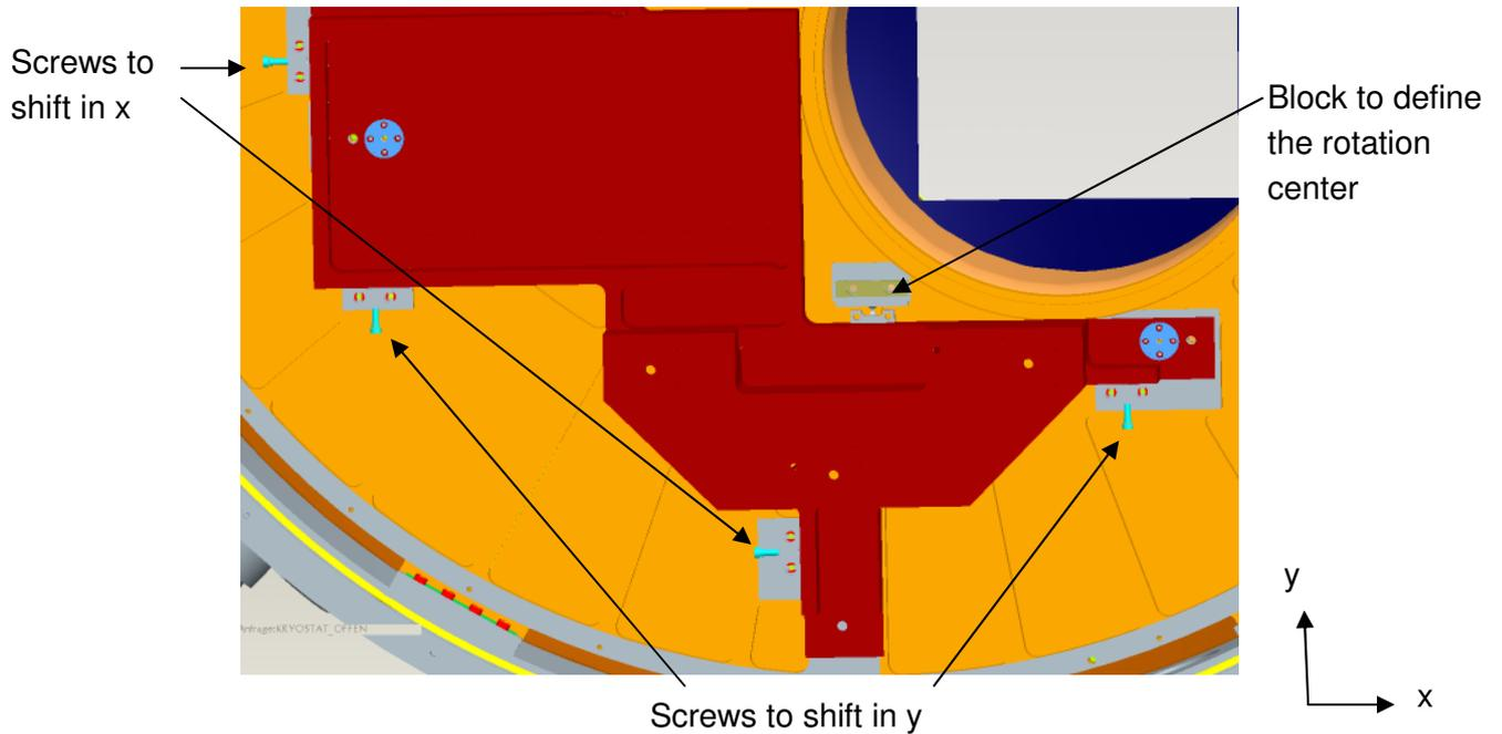
**Figure 18: Optics mount 1 adjustment principle**
