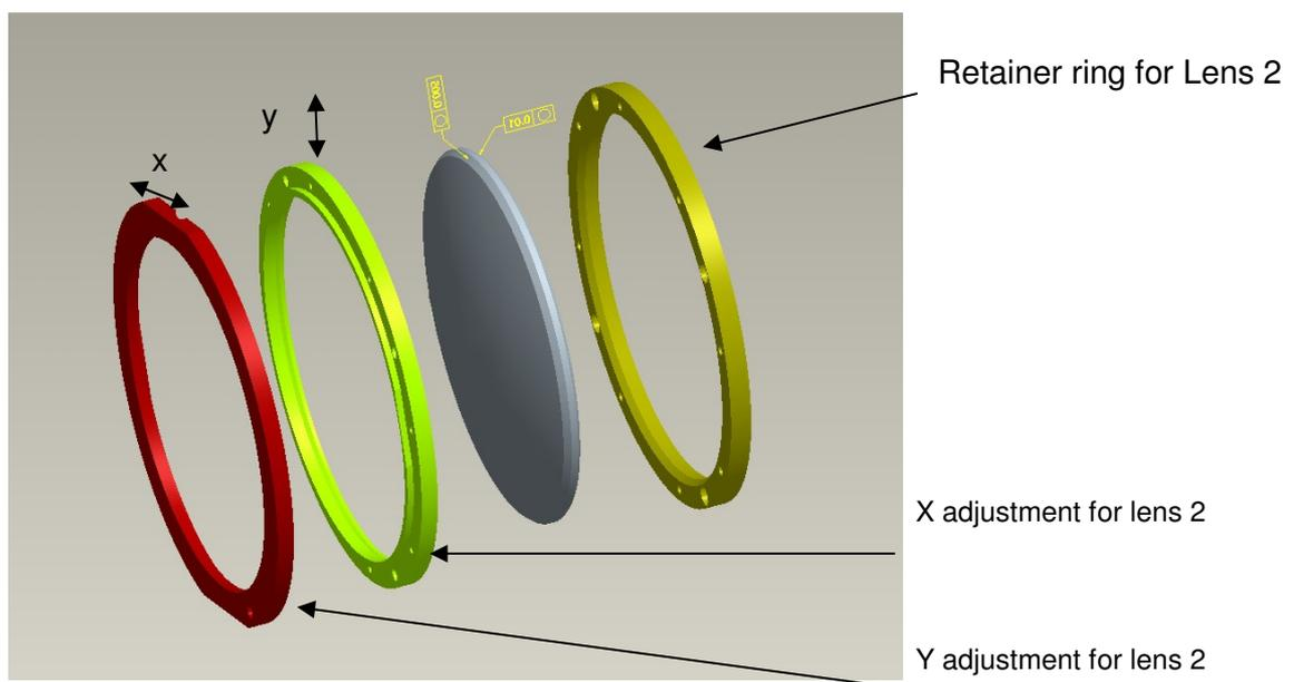
**Figure 27: Adjustment unit for Lens 2**
