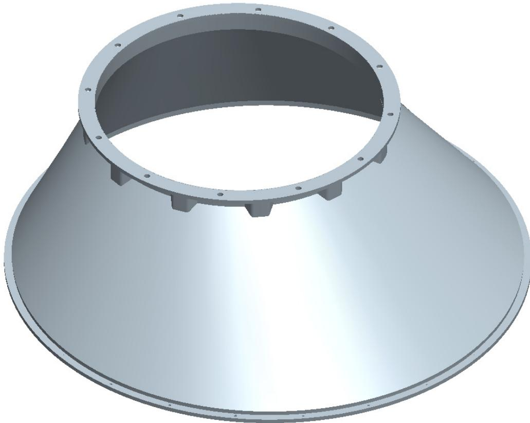
**Figure 65: Telescope Adapter**
