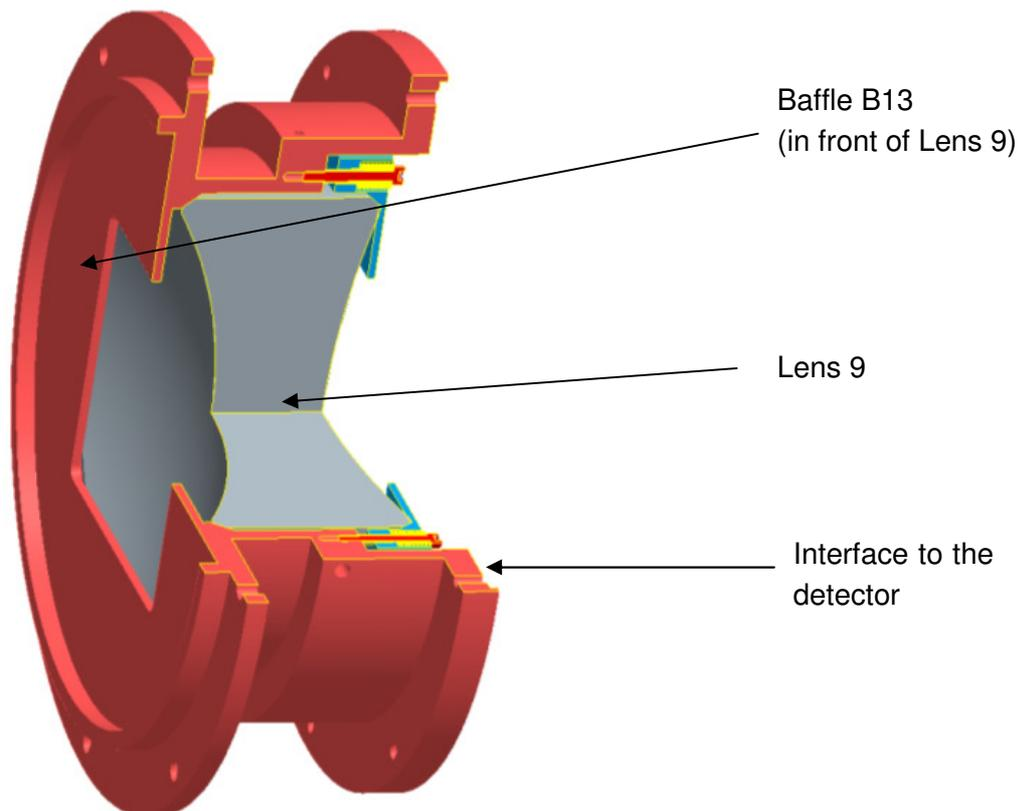
**Figure 39: Lens mount 4 with lens 9 attached.**
