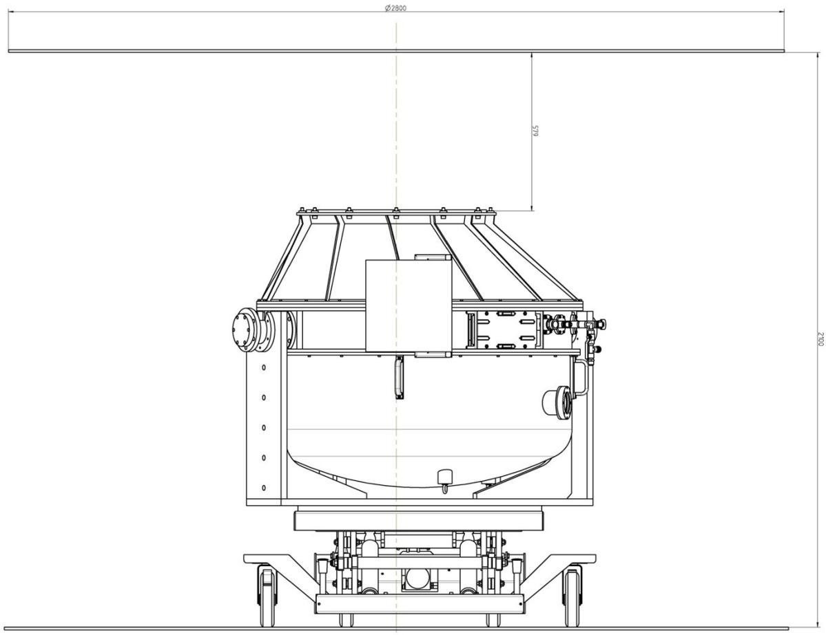
**Figure 79: PANIC with reference to the 2.2m-telescope instrument mounting flange**
