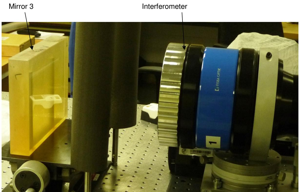
**Figure 80: The uncoated mirror 3 is tested with an interferometer before integration into its mount.**
