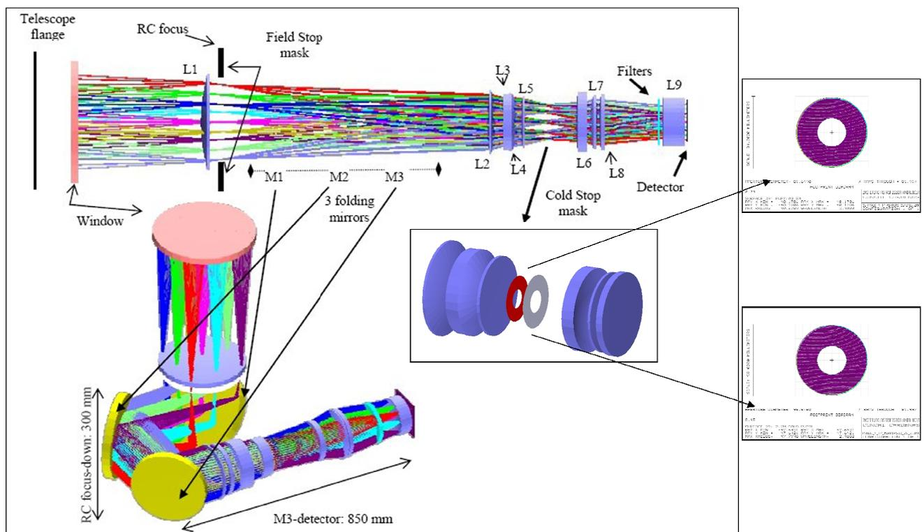
**Figure 2: PANIC optical layout, original (top) and folded (bottom)**
