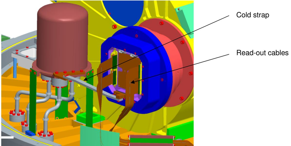
**Figure 71: Detector assembly**
