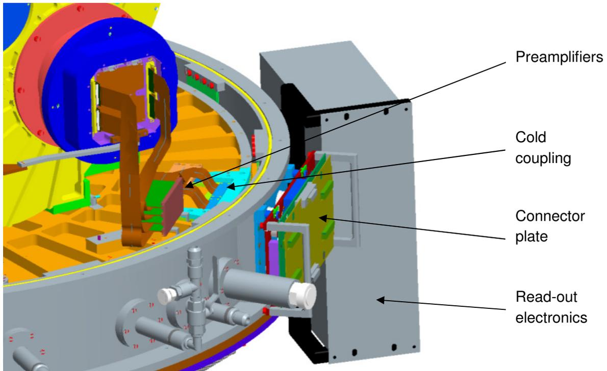
**Figure 72:Read-out cabling**
