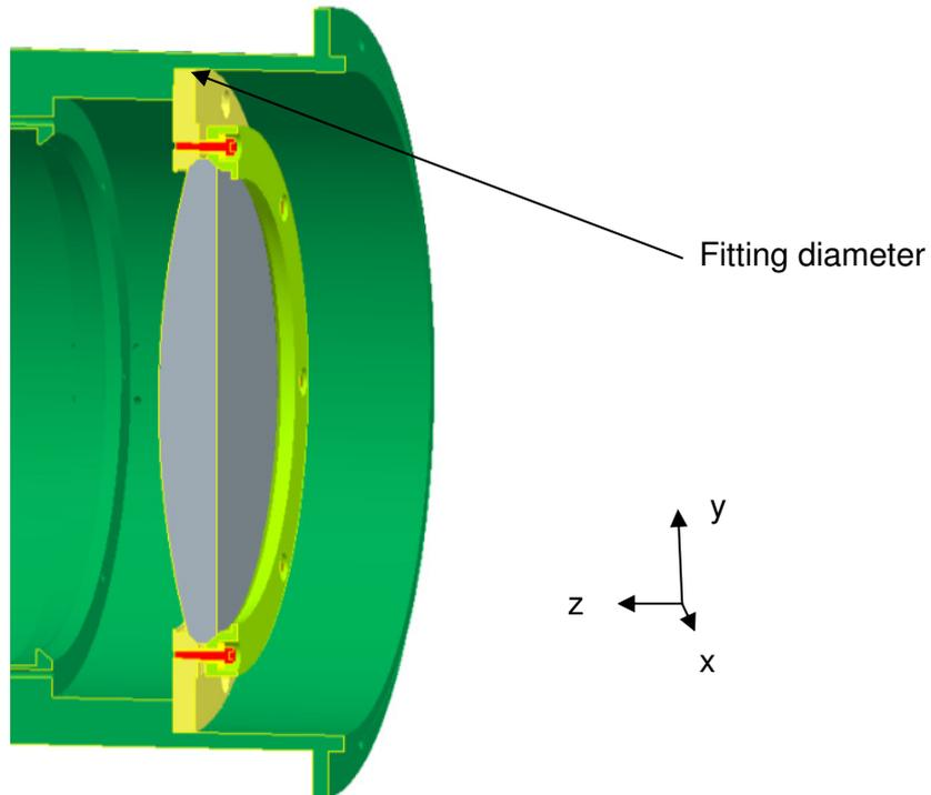
**Figure 29: Lens 5 with its support in lens mount 2**
