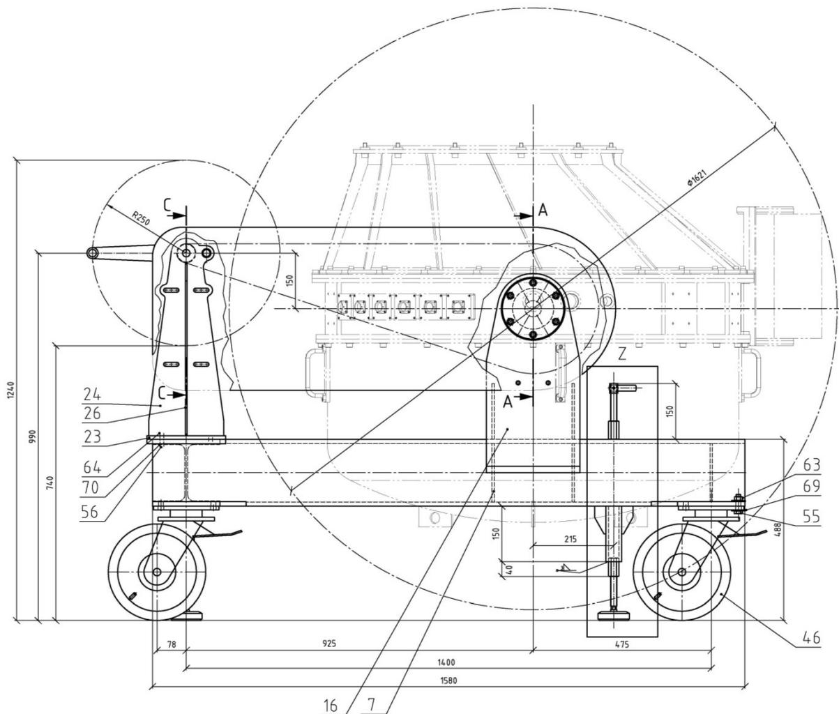
Figure 74: Dimensions of trolley A
