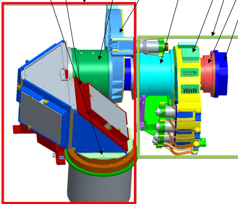
**Figure 9: Overview over the optical elements and their mounts**
