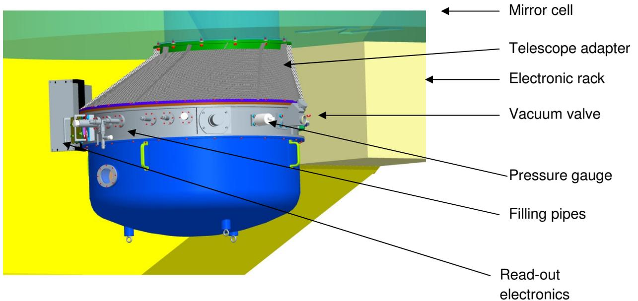
**Figure 5: PANIC at the 2.2m telescope**
