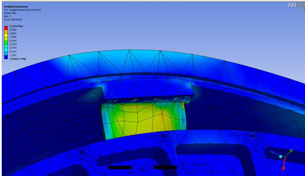
**Figure 54: Finite element simulation of the spacers**
