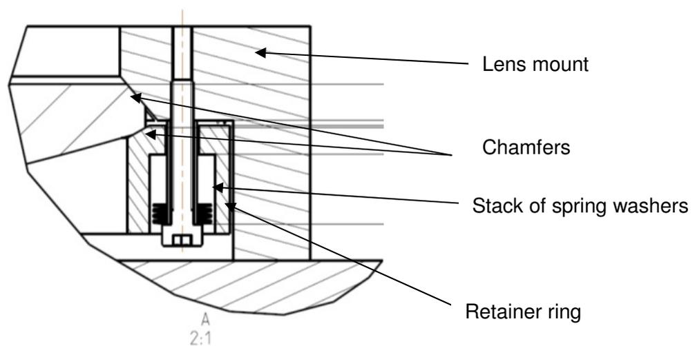
Figure 10: Cross-sectional view through the lens alignment design (explanation in the text)
