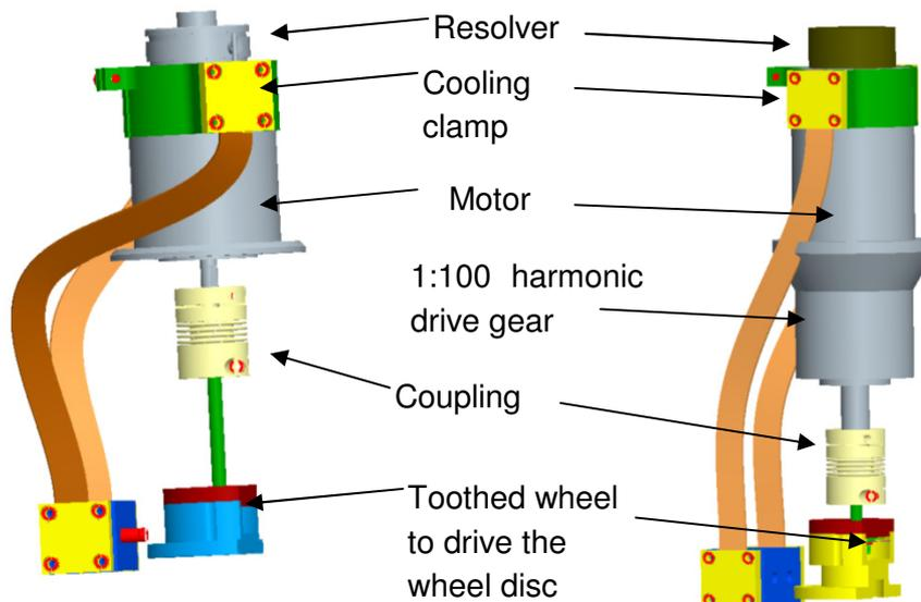
**Figure 42: The main parts of the wheel drives. Left: one of four identical filter wheel power trains, right: the power train for the cold stop wheel**
