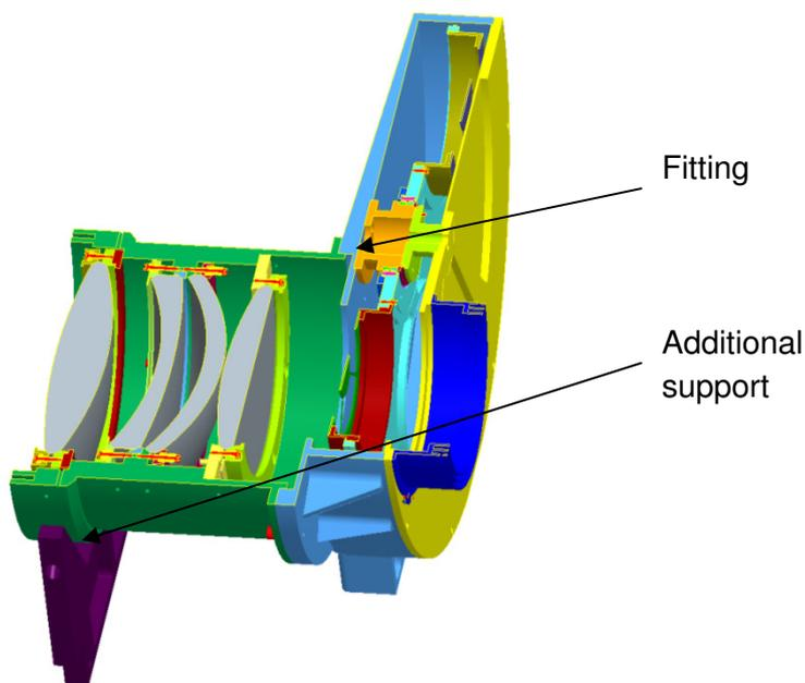
**Figure 26: Positioning of lens mount 2**
