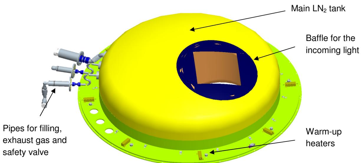
**Figure 48: The main tank subassembly**
