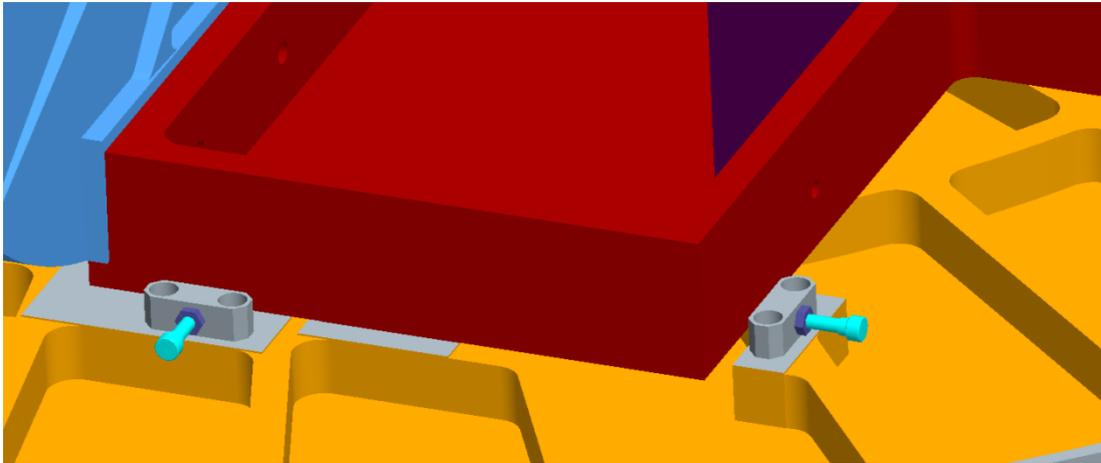
**Figure 17: Adjustment screws allow optics mount 1 to be shifted in x and y direction.**
