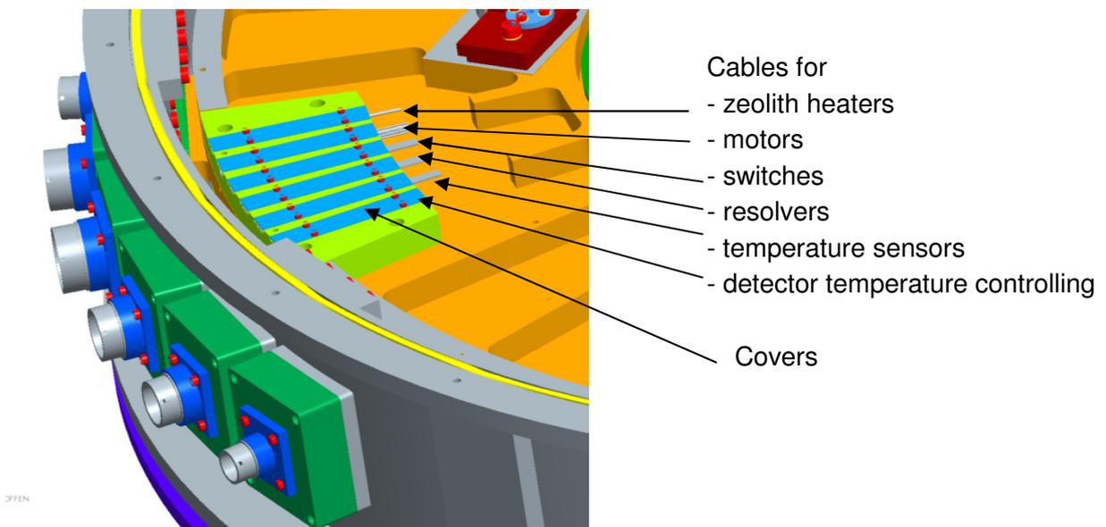
**Figure 55: Feedthroughs for the cryostat cabling**
