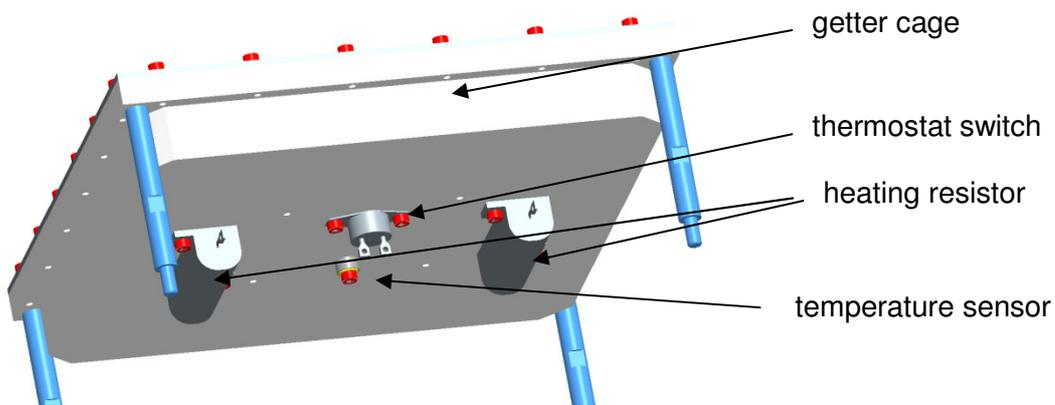
**Figure 59: Two heaters, a thermostat switch and a temperature sensor are used to control the temperature of the getter cage**
