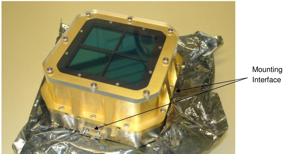
**Figure 68: The detector module as delivered from Teledyne**
