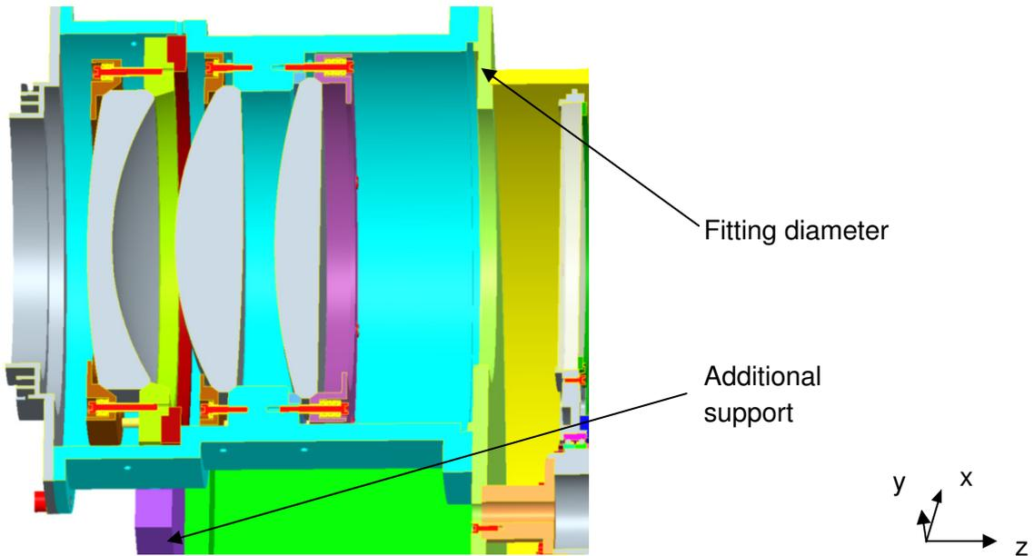
**Figure 33: Positioning of lens mount 3**
