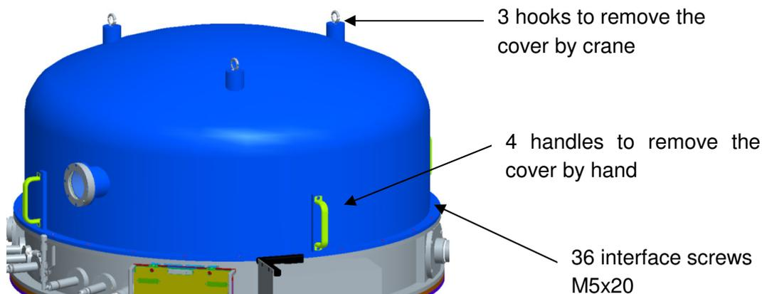
**Figure 60: removing the vacuum cover**
