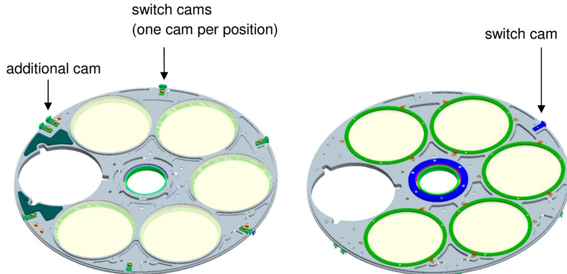
**Figure 44: The filter wheel disc front side (left) has one cam per position, the rear side (right) has only one cam.**
