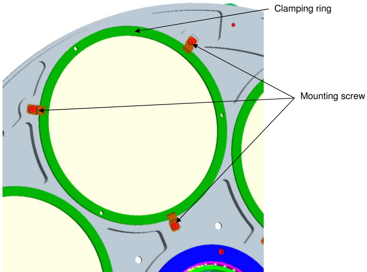
**Figure 38: Filter mounting elements**
