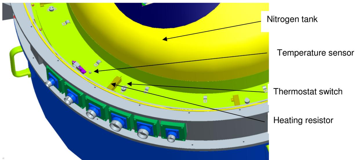
**Figure 58:** Eight heaters in two circuits attached to the nitrogen tank are used to warm-up PANIC
