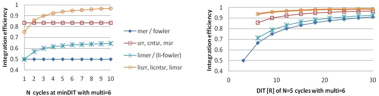
Figure 3: Integration efficiency of the multi correlated readout modes with correlation count  $\text{multi}=6$ , as exposure time ( $N \cdot \text{DIT}$ ) divided by the needed detector clocking time: On the left side drawn with minimal DIT versus number  $N$  of repeated cycles, on the right side drawn with  $N=5$  versus DIT in units of the single frame read time  $R$ .
