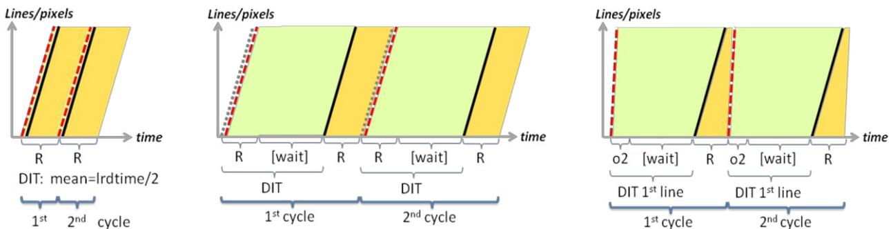
Figure 4: The left readout scheme shows the **rlr**, the middle scheme the **rr-mpia**, and the right the **o2scr** readout scheme.
