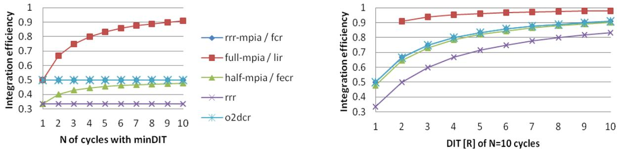
Figure 2: Integration efficiency of the double correlated readout modes, as exposure time ( $N \cdot \text{DIT}$ ) divided by the needed detector clocking time: On the left side drawn with minimal DIT versus number  $N$  of repeated cycles, on the right side drawn with  $N=10$  versus DIT in units of the single frame read time  $R$ .
