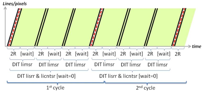
**limsr**, line interlaced multi sample read, uses exactly the same pattern scheme like the lisrr, but results in (multi/2-1) double correlated images.
