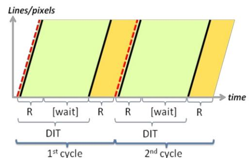
against the fecr, the fast end-of-line-reset correlated read. This persistence effect may appear at minDIT with bright sources in all readout modes, which show after each cycle the orange overflow time R (see also the overflow protection option).
