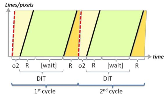
**rrr-mpia**, reset-read read of  $mpia$ , or **fcr**, fast correlated read, is based on the fast line reset and the single frame read  $R$  (see chapter 2.1).
