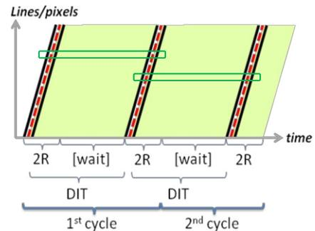
**half-mpia**, or **fecr**, fast end-of-line correlated read, is based on the fast line reset at the end of line clocking (see chapter 2.3).
