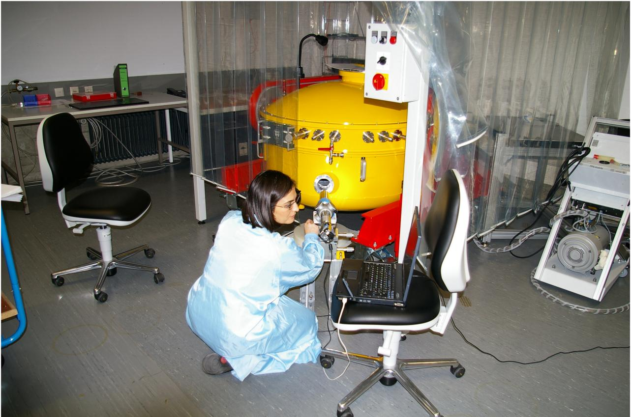
Figure 6: Checking the alignment of the camera at the PANIC's lab of the MPIA in October 2010.
