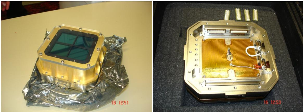
**Figure 3: The focal plane array. The greenish areas are the 4 light sensitive areas (left). The back of the module with connectors and heaters (right)**
